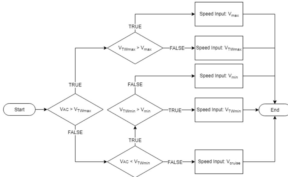
**Figure 3:** Flowchart of the generation of the speed input by the A-FMS
