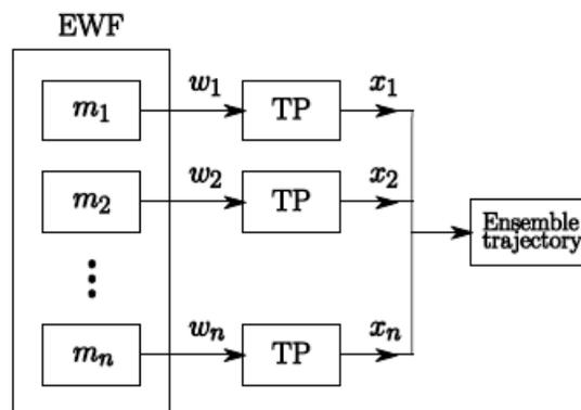
Figure 2.5: Ensemble trajectory prediction with  $m$  - member,  $w$  - weather,  $x$  - trajectory[14]
