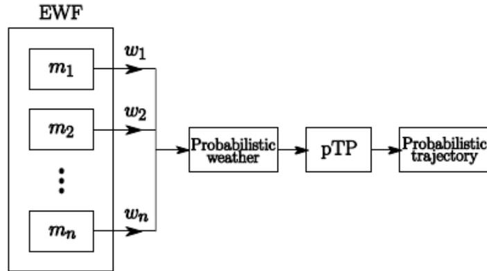
Figure 2.6: Probabilistic trajectory prediction with  $m$  - member,  $w$  - weather[14]
