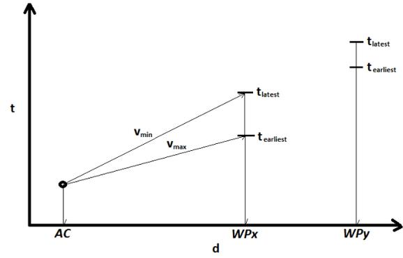
Figure 1: Graphical representation of the aircraft's trajectory
