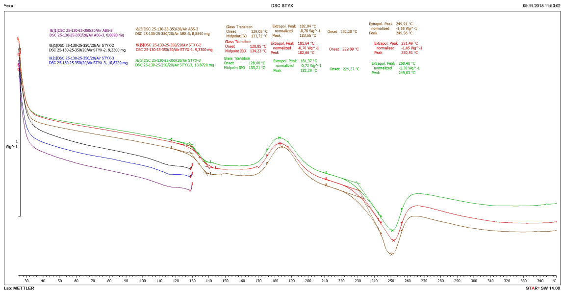
Figure B.3: DSC measurement of Nylon 12 (STYX) showing T_g at \approx 134^\circ C , an endothermic crystallization peak with onset at \approx 172^\circ C and exothermic melting well with onset at \approx 230^\circ C .
