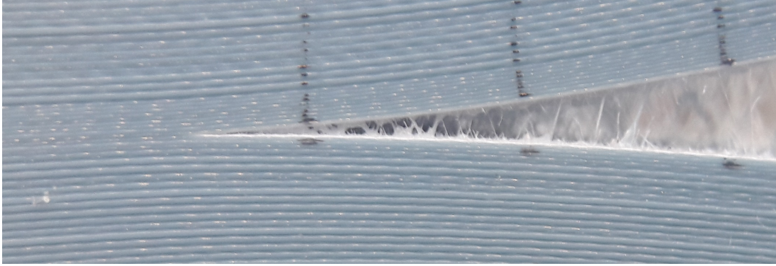
Figure 6.6: Figure showing the crack propagating in between printed layers, showing that samples used measure interlayer properties.
