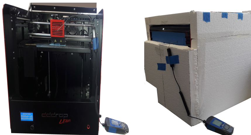
Figure 5.10: Photograph showing stock DDDROP set up (left) and the insulated DDDROP printer (right) capable of reaching controlled T_{env} up to 70^{\circ}\text{C} and the external thermocouple.
