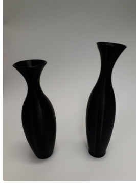
Figure 3.17: An as printed vase (left) and a similar vase after 30 minutes at T_g + 30^\circ C .
