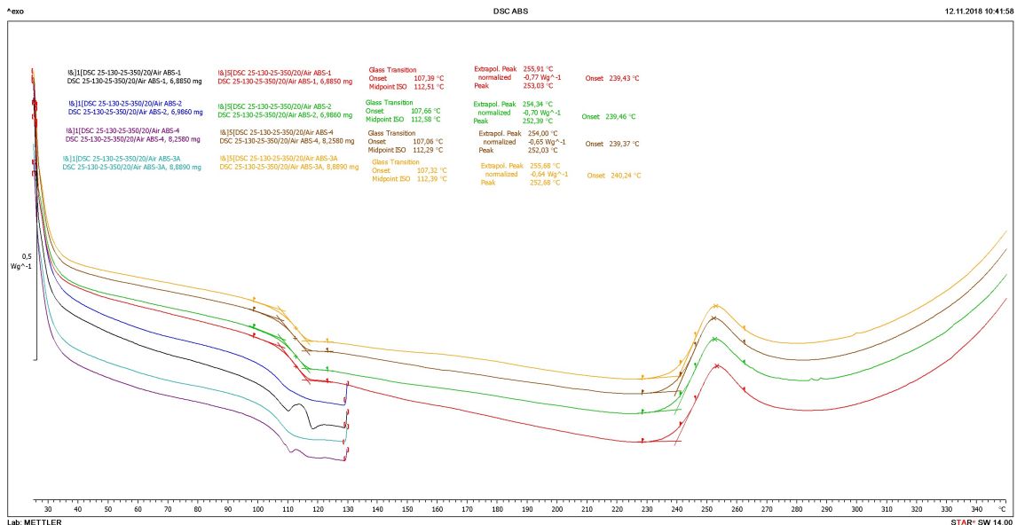
Figure B.1: DSC measurement of ABS showing T_g at \approx 112^\circ\text{C} and a presumable endothermic crystallization peak with onset at \approx 240^\circ\text{C} .
