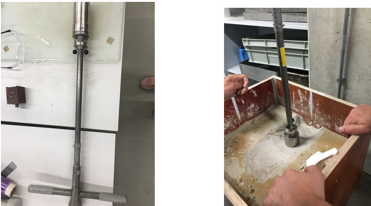
Figure A.15: The device used to take the core samples.
