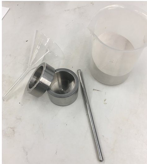
Figure A.13: The Equipment used for determining the minimum and maximum void ratio.
