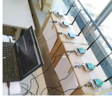
Fig. 2: Placement of receiver LoRa nodes at 22 m and 30 m altitude to perform CAD on different spreading factors.
