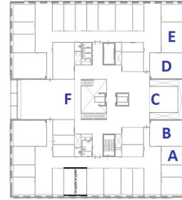
Fig. 12: Thirty devices distributed per five devices per group in six groups. Floor-plan of building with group-positions according to their SF. Gateway positioned with group C.
