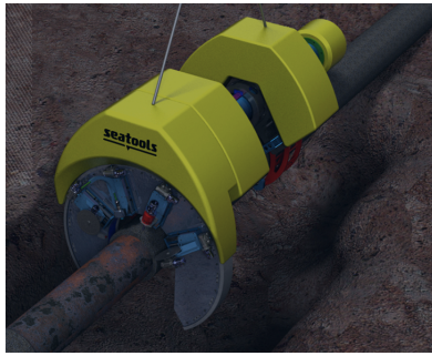
Figure 4.5: The concept of the coating removal tool by Seatools BV. image from seatools.com
