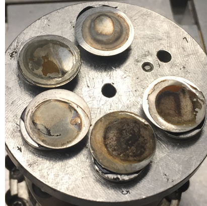
Figure 6.15: Several samples after treatment after removal of the corrosion product
