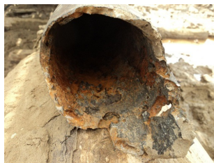
Figure 4.3: A severe case of \text{CO}_2 -corrosion on a steel pipeline, image from http://himipex.com/
