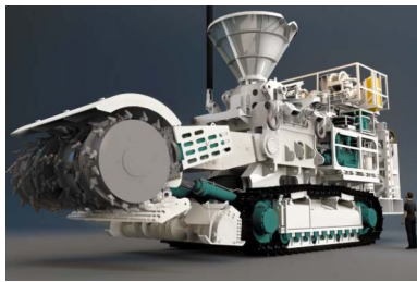
Figure 4.6: An impression of a deep sea bulk-cutter. Image from ethicalmetalsmiths.org
