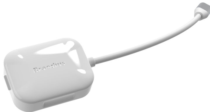
Figure 34: Probe design. A short wire with an external female connector is attached to the probe to save room inside the housing and for a more manageable solution (e.g. a long cable that is permanently attached to the probe).
