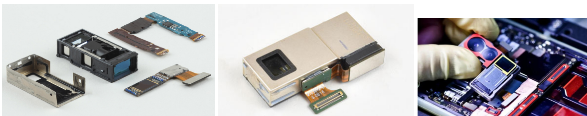
Figure 24: Compact camera module containing the sensor, optics and focus mechanism.
