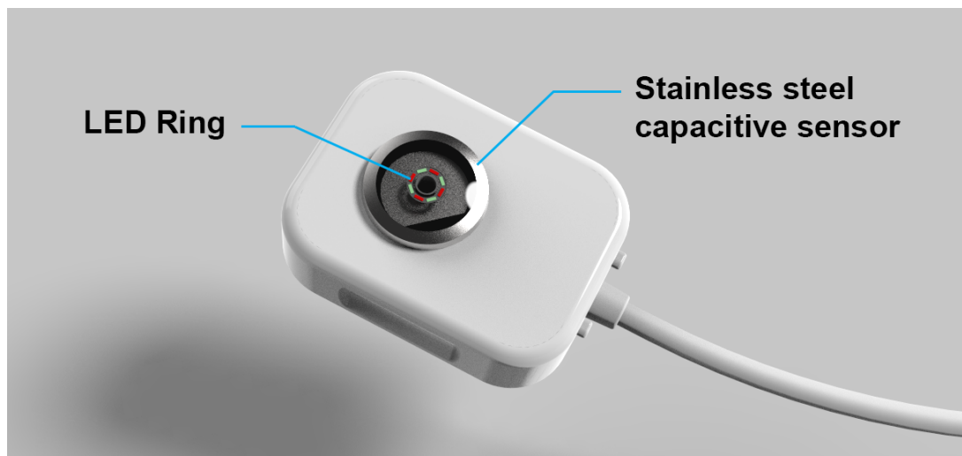
Figure 35: Underside of the probe. The LED ring can have two or more types of LEDs to target e.g. the oxygenated and deoxygenated state of haemoglobin. The edge of the glass dome has a stainless steel ring connected to a capacitive touch sensor. This allows for pressure feedback. When it comes into contact with the patient's skin, it will notify the user too much pressure is applied.
