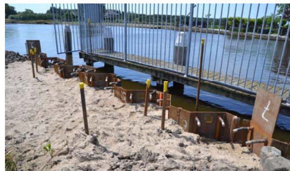
Fig 8. Test set-up of the energy sheet pile wall near Delft, the Netherlands
