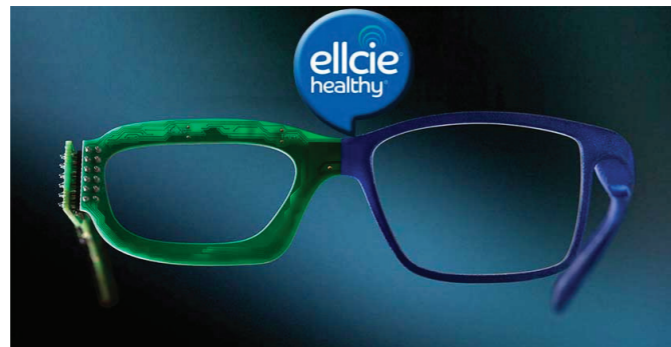
Figures 3.8 and 3.9: The eSkin Sleep and Lounge smart pyjamas by Xenoma and the smart connected eyewear by Ellcie Healthy.
