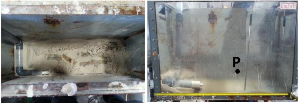
FIGURE 5.8 LEFT, TOP VIEW OF THE AQUARIUM, RIGHT FRONT VIEW OF THE AQUARIUM WITH NOZZLE AND CONDUCTIVITY PROBES; P REFERS TO THE LOCATION OF THE PRESSURE SENSOR.
