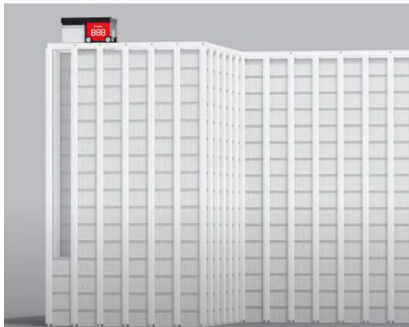
Figure 3.6: AGVs riding on top of a warehouse rack with a grabbing mechanism that can reach the last crate
