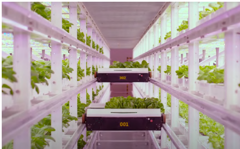
Figure 3.3: Inside view of the SANANBIO's vertical farm with an empty middle row for an automated guided vehicle (AGV) [5].
