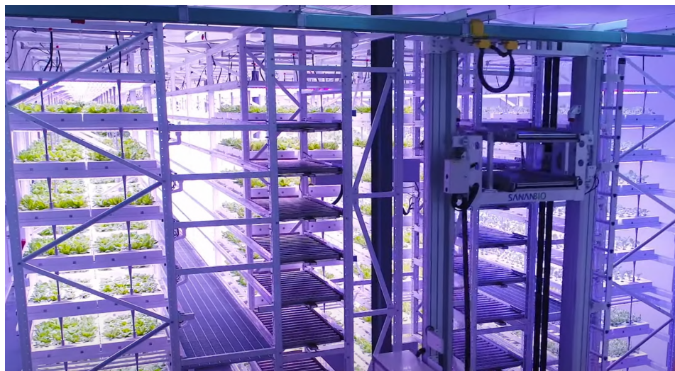
Figure 3.4: Front view of the SANANBIO's vertical farm with a 2D shuttle
