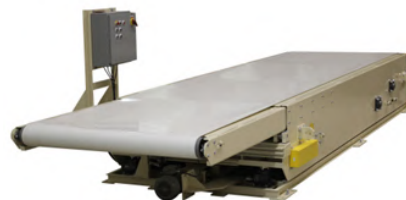
Figure 5.2: An extendable conveyor belt to cover the gaps between the cell and the lift as well as between the lift and the conveyor.
