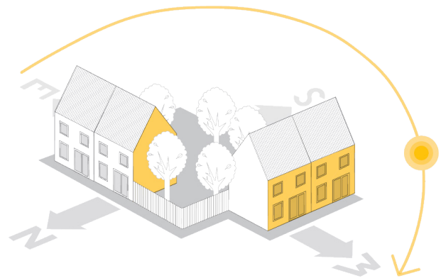
Figure 5.5 Westward orientation of the building with large glazing will cause the solar gain late in the evening with high outdoor temperatures. Source: NHBC,2012
