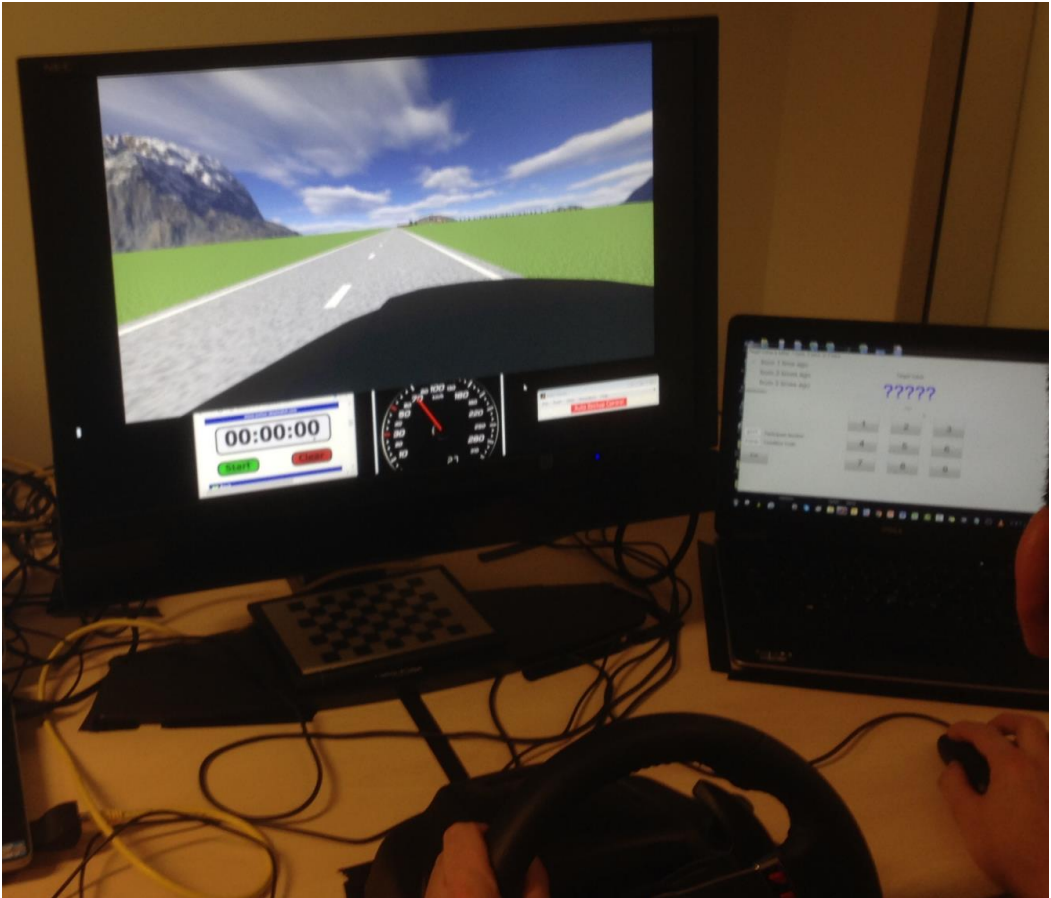
Figure 4.2.1. Driving simulator arrangement including a gaming steering wheel attached to the edge of the table (bottom), floor pedals (not shown), driving simulation visuals displayed on a monitor (middle), and secondary task on a laptop with an external mouse (right).
