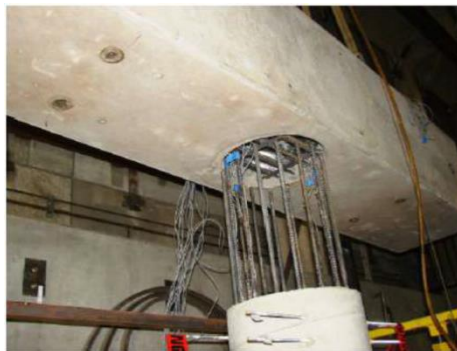
Figure 3.12: Principle of connecting the reinforcement bars to the cap (NCHRP (2011)).
