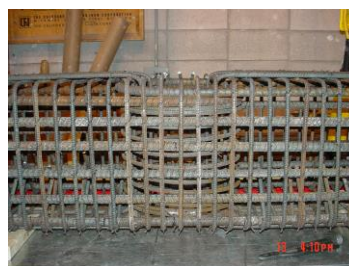
Figure A.5: Third option with at the top the U-shaped bars (Stephens et al. (2005)).
