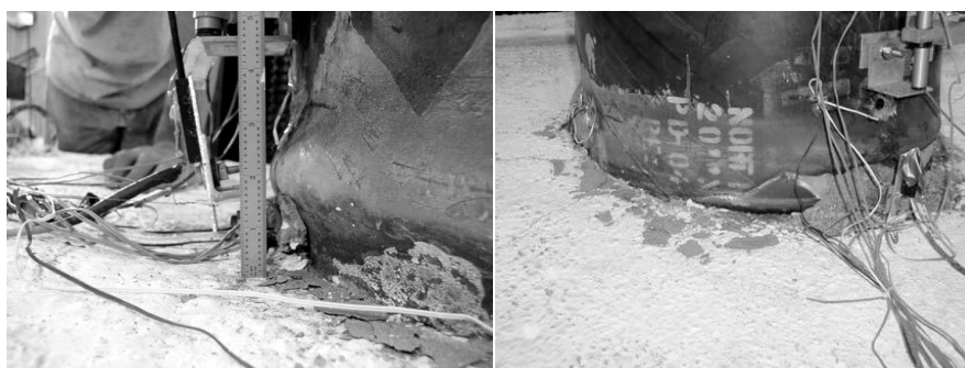
Figure 3.1: Local buckling of the pipe piles on the left and tearing of the tube at the position of the local buckle at the right (Stephens et al. (2014)).
