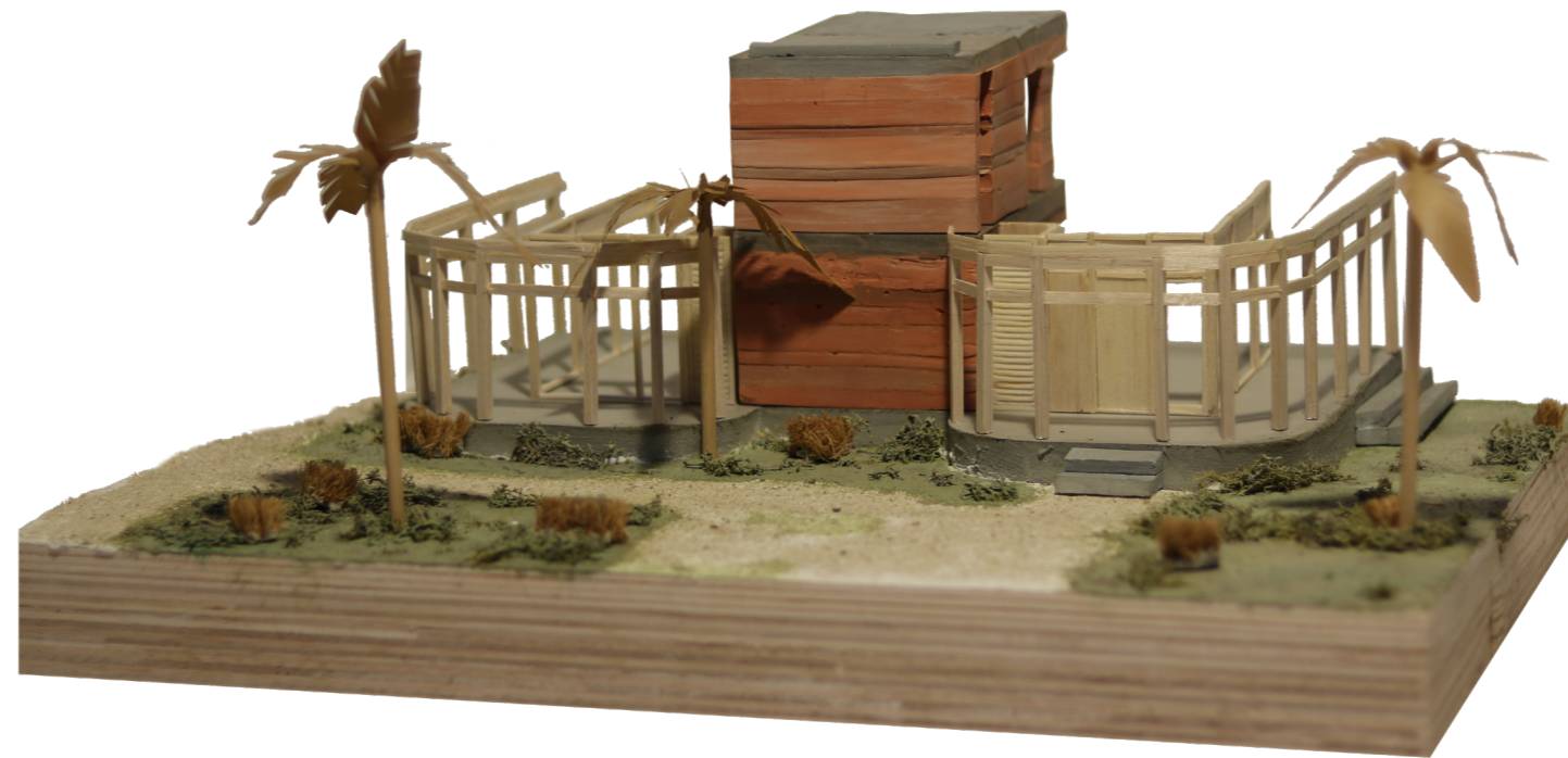
rammed earth walls with concrete ringbeam rammed earth walls build with excavated clay loam soil.
