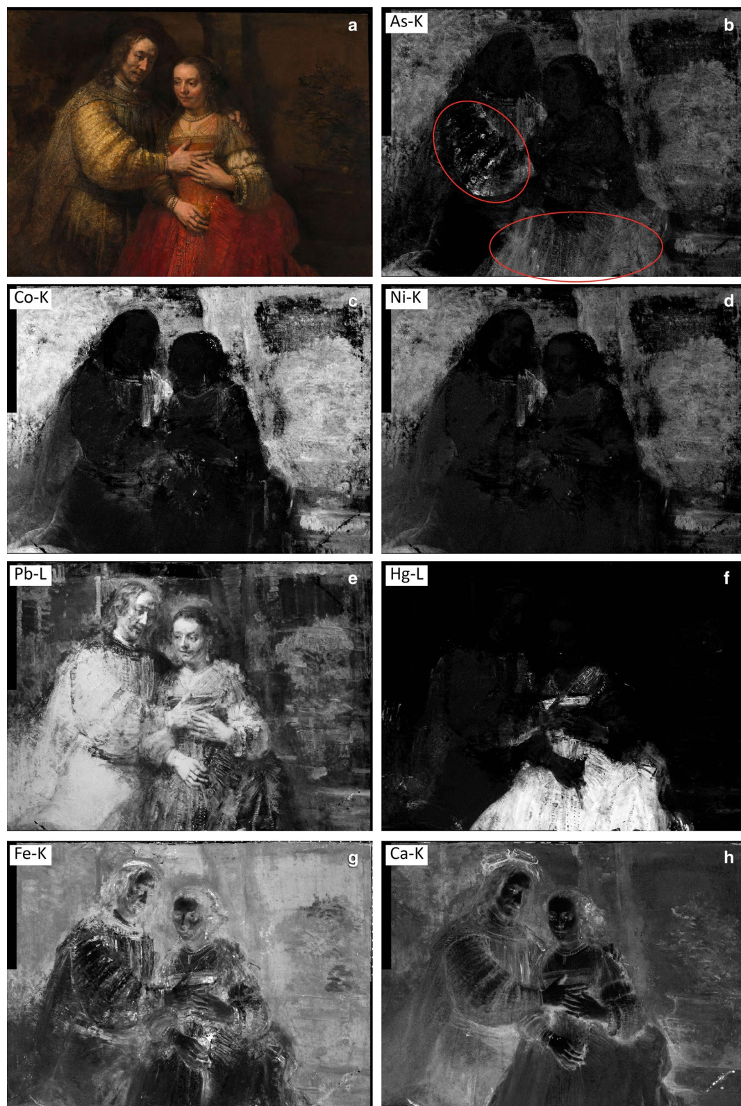
Fig. 1 Rembrandt, Portrait of a Couple as Isaac and Rebecca, known as 'The Jewish Bride' , c. 1665, oil on canvas (lined), 121.5 × 166.5 cm, Rijksmuseum Amsterdam (SK-C-216). Visible light image ( a ), and corresponding MA-XRF maps: arsenic ( b ), cobalt ( c ), nickel ( d ), lead ( e ), mercury ( f ), iron ( g ), calcium ( h )
