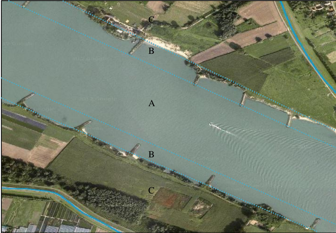
Figure 2.1: River Waal during low discharge with (A) main channel, (B) groyne fields and (C) floodplains marked, source: Google Maps.
