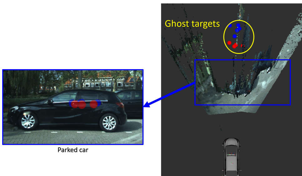
Figure 2.13: Real world examples of ghost targets. On the left, targets are projected into the camera view. On the right is a top view of the scene with the stereo camera point cloud. Notice that the targets are farther away from the ego-vehicle (bottom of top view) than the parked car. This is because the radar signal is reflected off the large flat side of the parked car, and the radar sensor is detecting the ego-vehicle itself. The colors of the targets indicate the outcome of the classification algorithm presented in Chapter 5. Namely, blue targets have the car class assigned to them, red targets have the cyclist class assigned to them.
