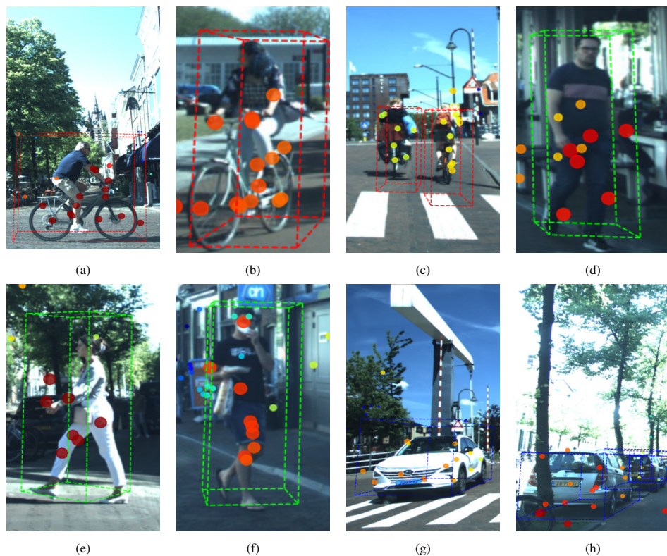
Figure 6.7: Examples of correctly detected objects by PP-radar projected to the image plane. Car/pedestrian/cyclist detections are shown as blue/green/red bounding boxes. Dots are radar targets colored by distance from the sensor.
