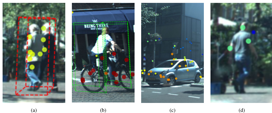
Figure 6.8: Examples of incorrect detections by PP-radar : (a) merged smaller objects (two pedestrians are detected as a single cyclist), (b) larger objects split into smaller ones (one cyclist is detected as two pedestrians), (c) strong reflections and clutter nearby (metal poles and high curbs) and (d) distant objects with too few reflections (far away pedestrian).
