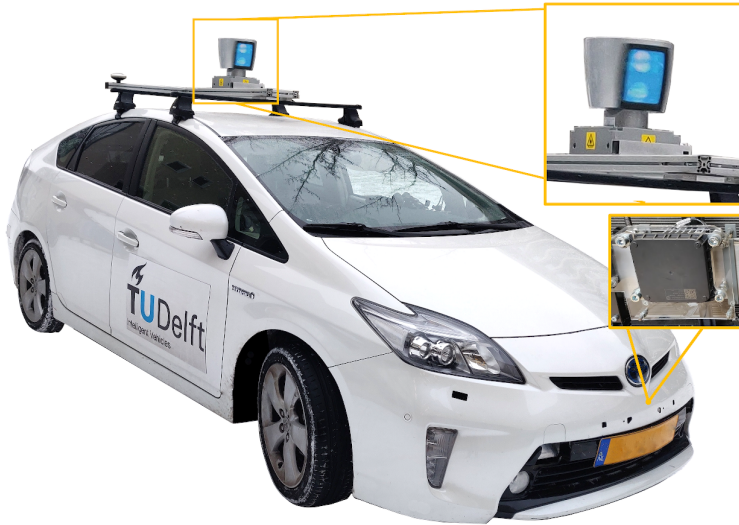
Figure 2.11: Demonstration of the possible placement of sensors in an intelligent vehicle. The scanning LiDAR sensor requires space to rotate to cover its field of view. Therefore, they are often placed on the roof of research vehicles or robot taxis. Radar sensors, on the other hand, can penetrate the plastic material of the bumper and can therefore be mounted (and hidden) almost anywhere on the vehicle.
