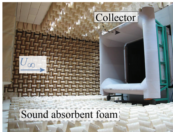
Figure 2.11: Anechoic test section of the DNW-NWB wind tunnel, in Braunschweig. Adapted from [30].
