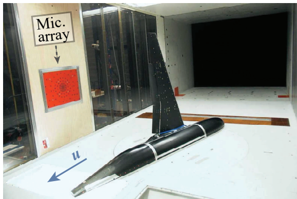
Figure 2.12: Closed test section aeroacoustic testing of an aircraft model, at DNW-LST wind tunnel. Adapted from [78].
