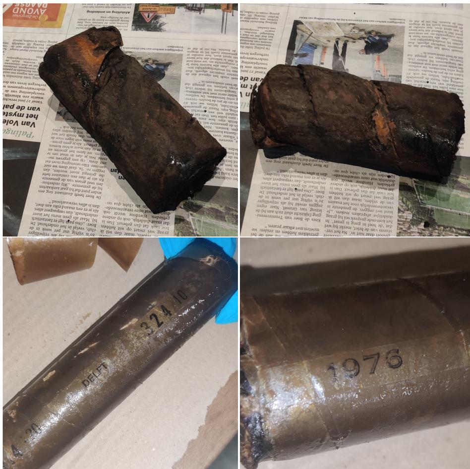
Figure C.1: Overview of the used PLC cable with its cable tag and manufacturing year.
