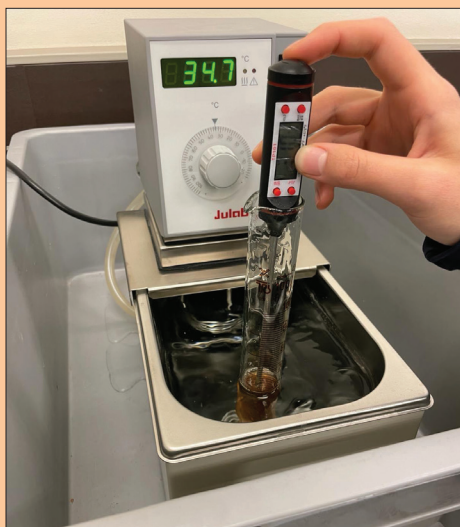
Fig. 1. A water bath was used to heat the honey uniformly.
