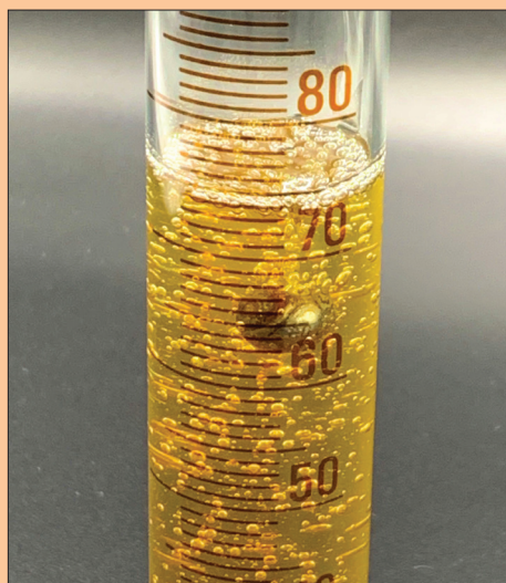
Fig. 2. The ball falling through the honey. Video analysis was used to determine its terminal velocity.
