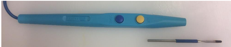
Figure 32: Monopolar electrosurgical knife (Reliant). Various blades can be attached to the knife, for this experiment the blade in the figure was used.
