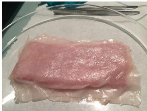
Figure 43: Specimen used for the experimental setup in Chapter 9, 10 and 11. Layers of adipose tissue with a thickness of 0.4mm on top of muscle tissue with a thickness of 1.5cm.
