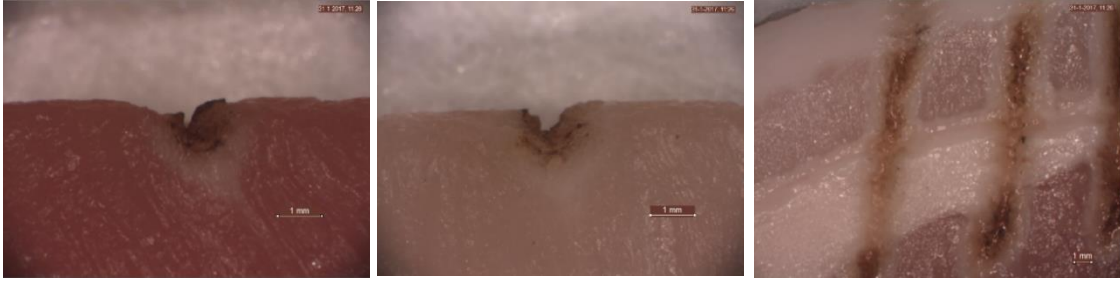
Figure 38: Section of coagulated pork muscle pork belly tissue (left) and adipose pork belly tissue (middle). On the right, a top view of coagulated pork belly tissue (2x). The coagulation is present in the muscle and the adipose tissue.
