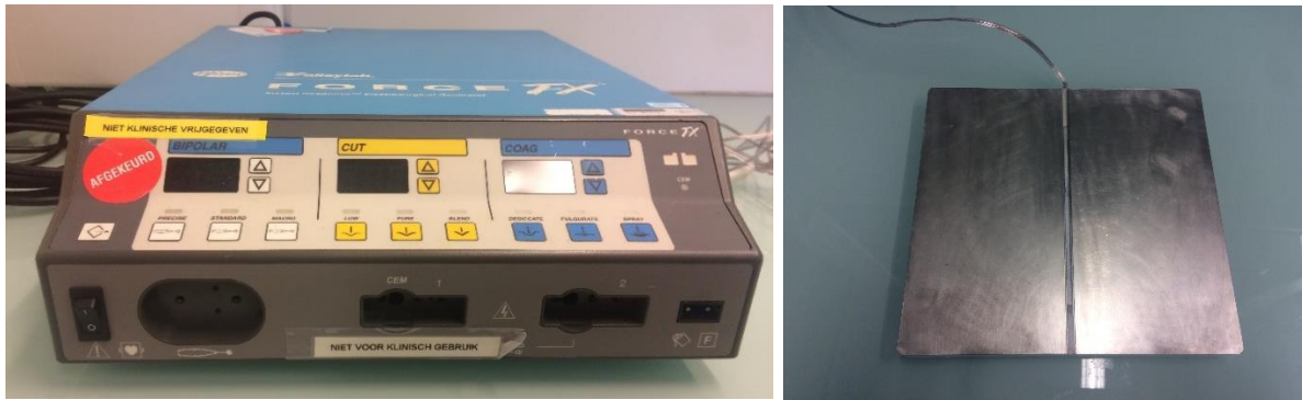
Figure 22: Left: Electrosurgical unit available at Philips In-Body Systems, which was used for the experiments described in this master thesis. Right: Dispersive pad which is used to transfer the current back to the electrosurgical unit.
