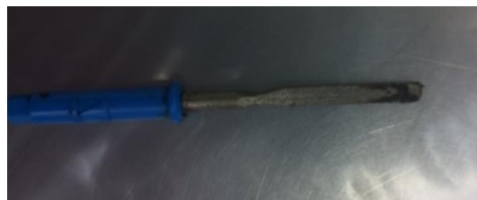
Figure 26: Ablation present on the electrocautery knife after the surgery.
