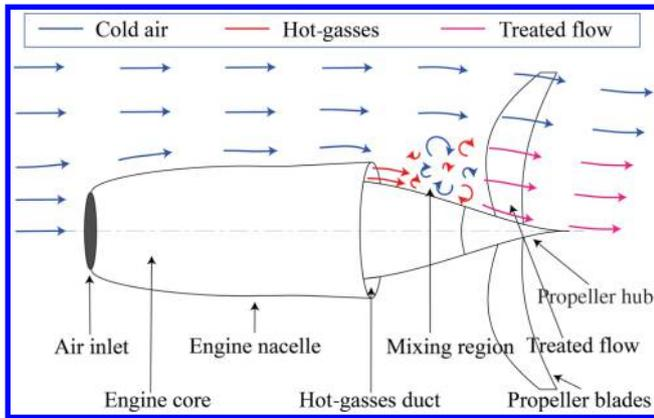
Fig. 1 Schematic of the *GasProp* concept for a turboprop engine in pushing configuration and qualitative thermofluid dynamic evolution of the flow around it.
