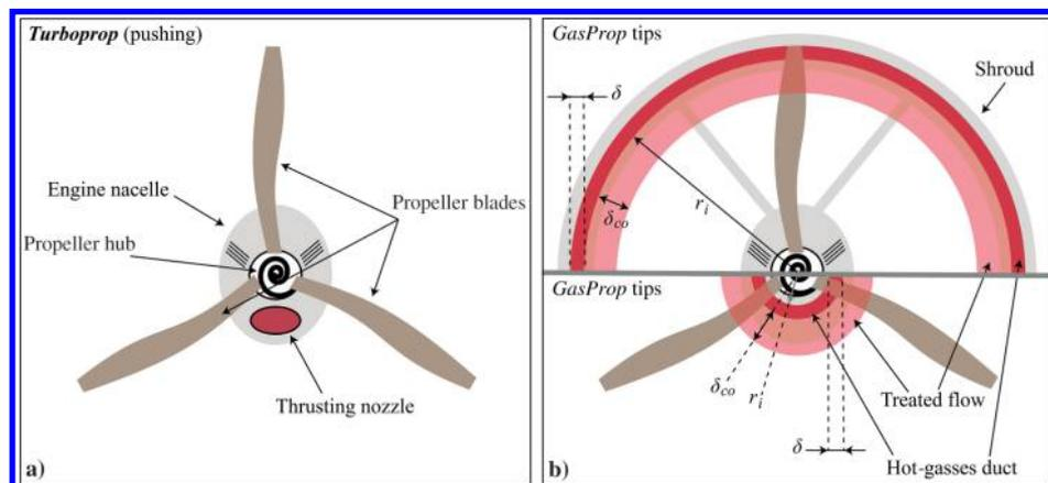
Fig. 2 Qualitative schematic of a common turboprop in a pushing configuration (Fig. 2a) and of the *GasProp* concept applied to the blades tip (Fig. 2b, top) and root (Fig. 2b, bottom) region. All views are from downstream.
