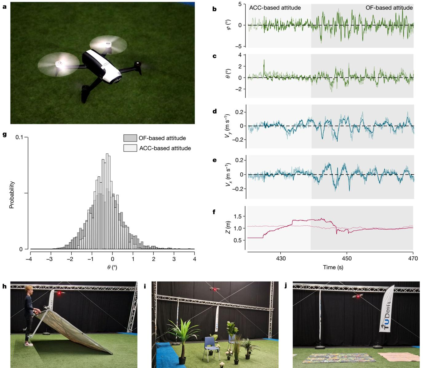
**Fig. 2 | The theoretical findings are confirmed by robotic experiments in which fully autonomous flight is demonstrated based on optic flow and gyro measurements.** **a**, Quad rotor robot used in the experiments.
