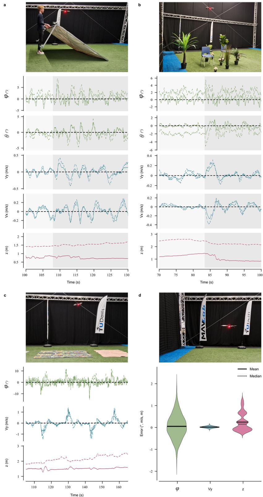
**Extended Data Fig. 1 | Robustness experiments robotic flight.** **a**, Quadrotor flying based on optic flow above a strong slope, which is dragged away, violating the assumption of a static flat ground. From top to bottom, the plots show the estimated attitude angles, velocities, and height. **b**, Quadrotor flying above three-dimensional objects, with artificial plant leaves moving due to the propellers' downwash, again violating the assumption of a static flat ground.
