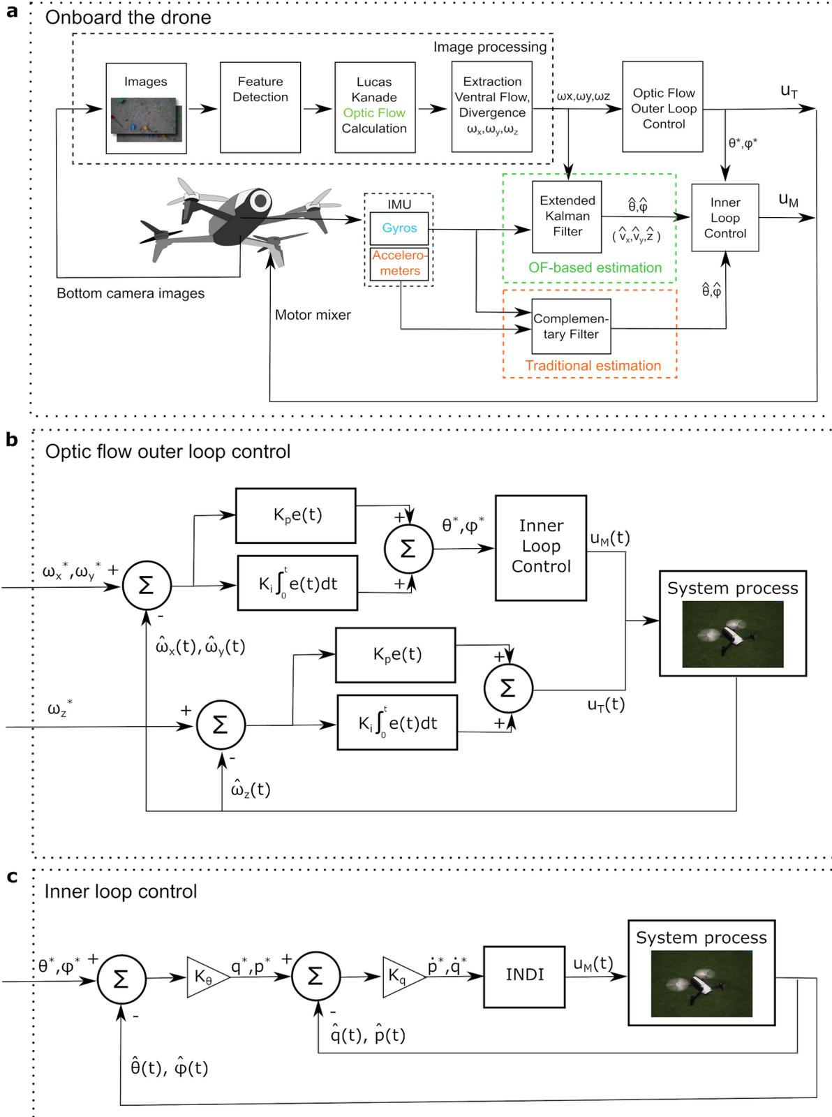
**Extended Data Fig. 4 | Processing and control loops onboard of the quadrotor drone (a Parrot Bebop 2) used in the robotic experiments.** **a**, Onboard image processing, state estimation, and control used for fully autonomous flight of the drone. **b**, Control diagram for the optic flow outer loop control, where the longitudinal and lateral optic flow  $\omega_x$  and  $\omega_y$  are used to
