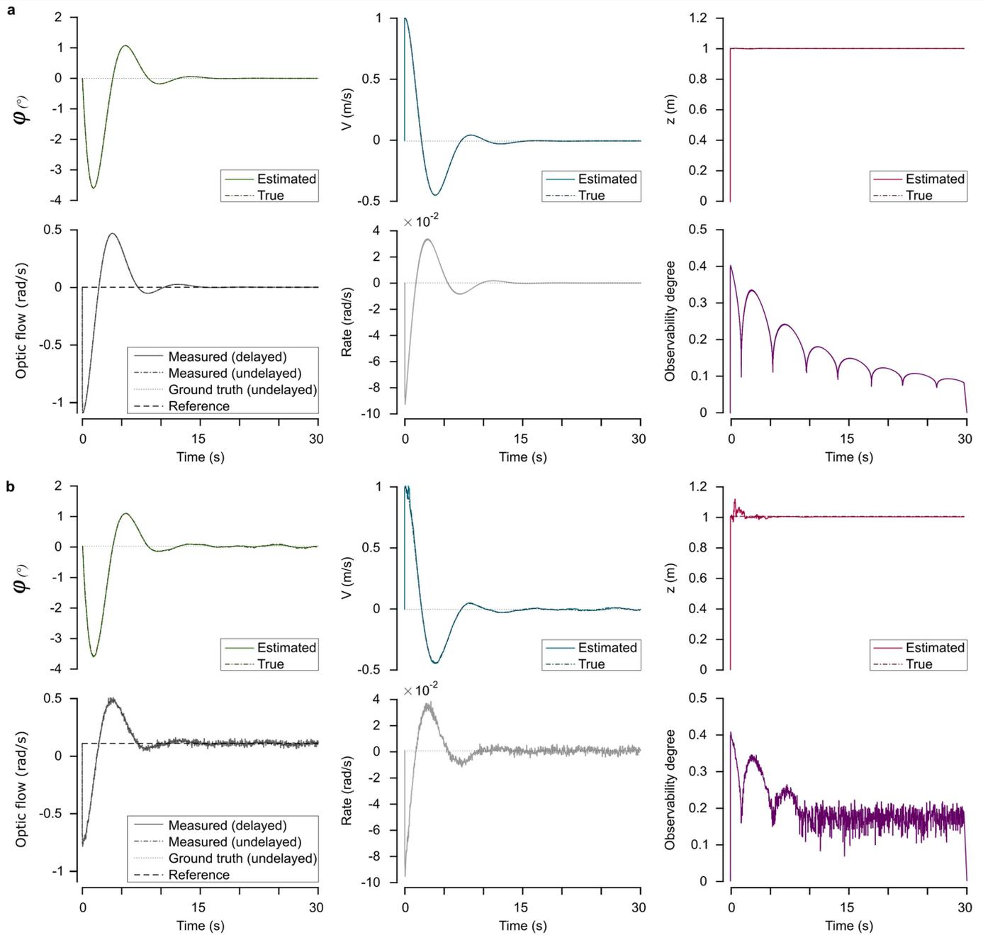
**Extended Data Fig. 7 | Simulation experiments to verify the stability proof-1. a**, Simulation without noise. Top row: The three states (true, solid line, and estimated, dashed-dotted line) over time. The dotted line indicates zero. Bottom row, from left to right: The optic flow  $\omega_y$  (solid line) and the reference desired flow (dashed line), the rate (solid line) with a dotted line at zero, and the
