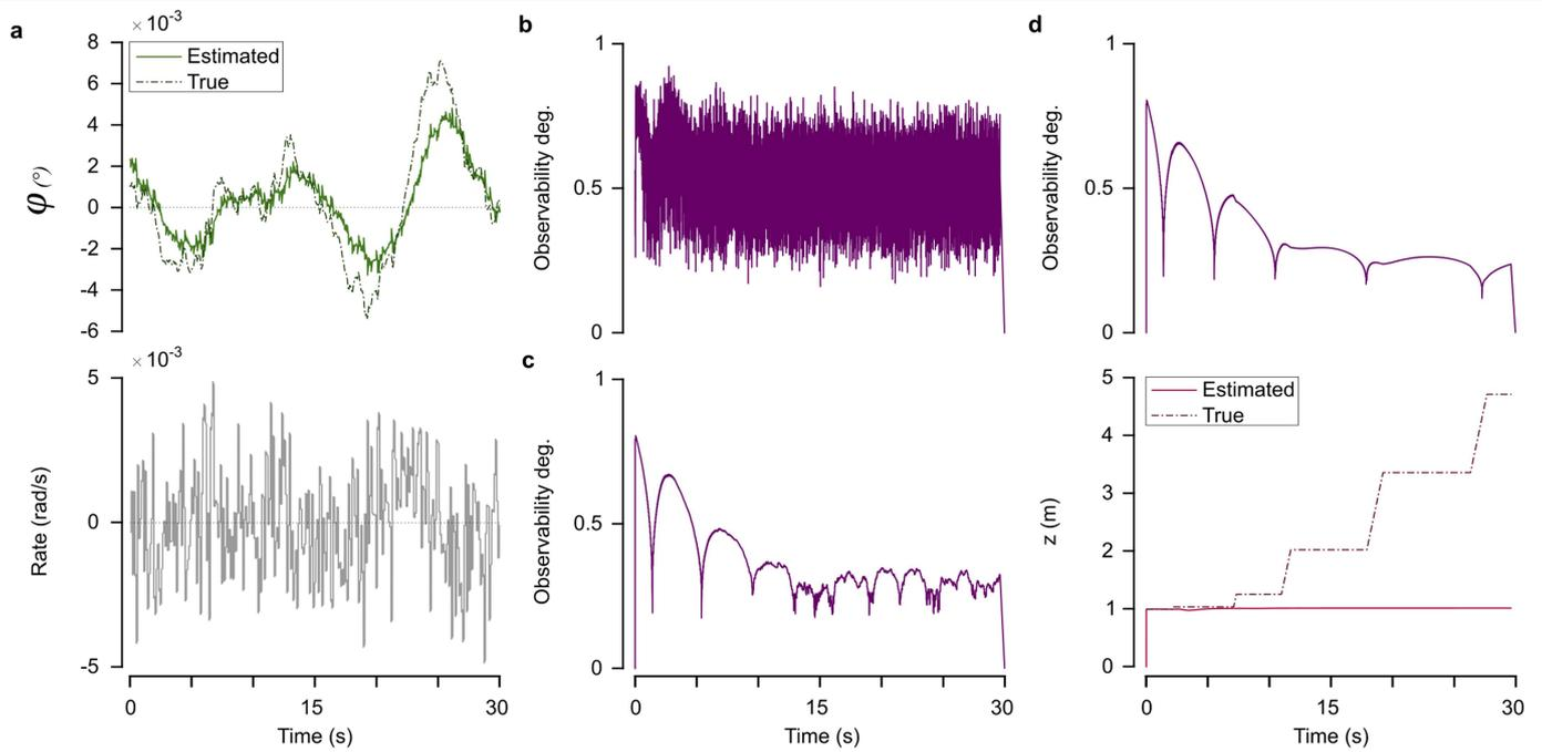
**Extended Data Fig. 8 | Simulation experiments to verify the stability proof-II.** **a**, Zoomed in view on time interval [15,25] seconds for a simulation with sensor noise. Top: True (dashed) and estimated (solid) roll angle over time. Bottom: roll rate. **b**, Observability degree over time for an experiment with
