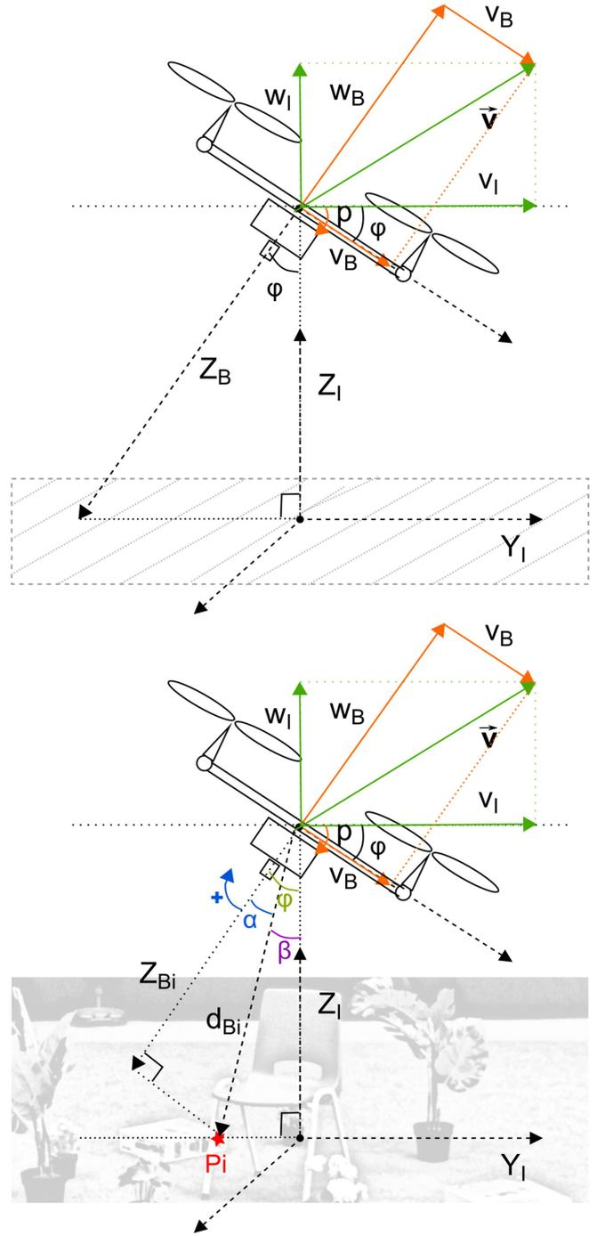
**Extended Data Fig. 3 | Sketches of different quad rotor and environment models.** a, Axis definitions for a constant height quad rotor model.  $B$  indicates the body frame, whereas  $I$  indicates the inertial frame. The arrows for  $Y$  and  $Z$  point into the positive directions. The attitude angle  $\phi$  represents the quad rotor's roll angle, and  $p$  the roll rate. The shaded rectangle represents the
