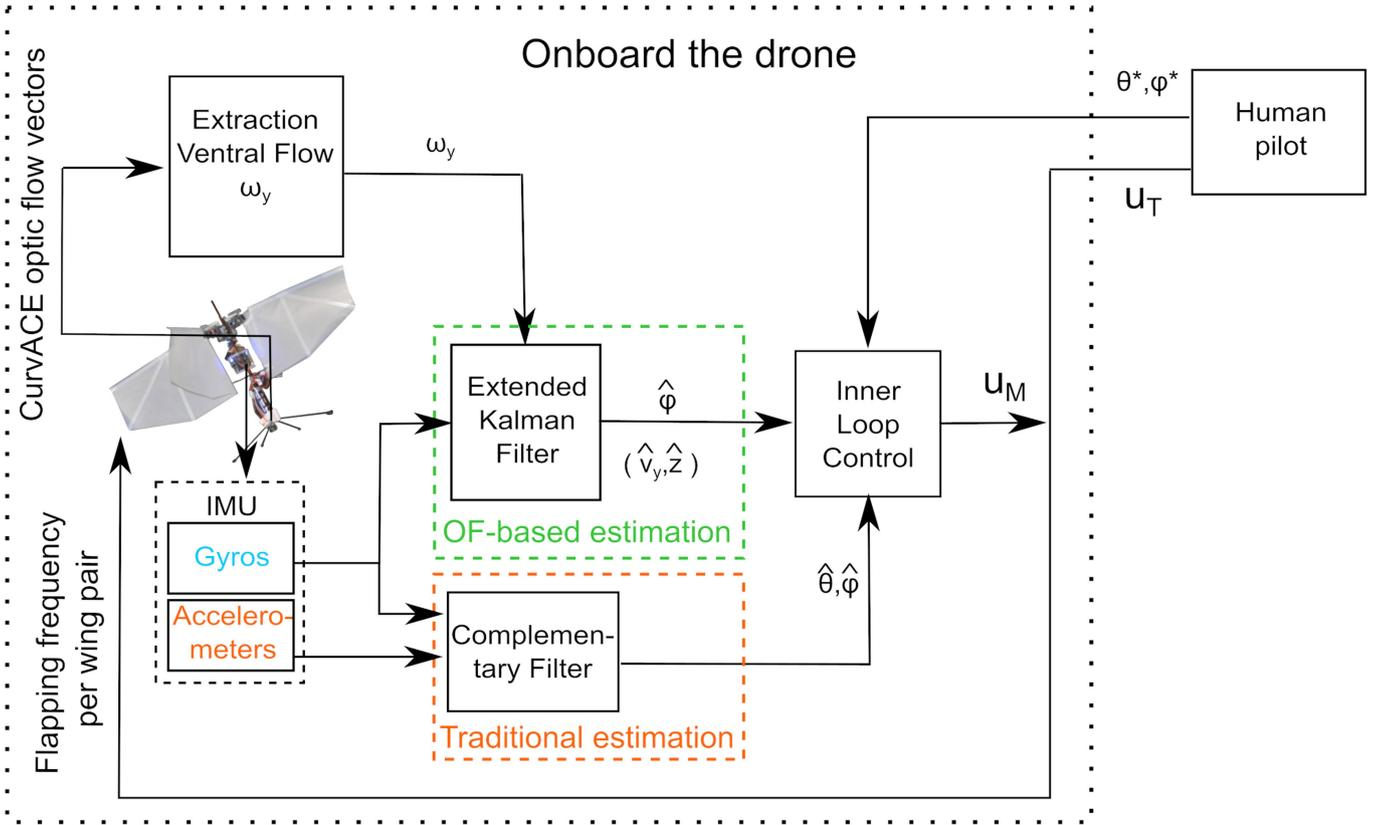
**Extended Data Fig. 5 | Setup of the robotic experiments with the flapping wing drone (a modified Flapper Drone).** A human pilot executes the outer loop control, while the drone itself runs the inner loop attitude controller, based on the onboard roll angle estimates. See the text for details.
