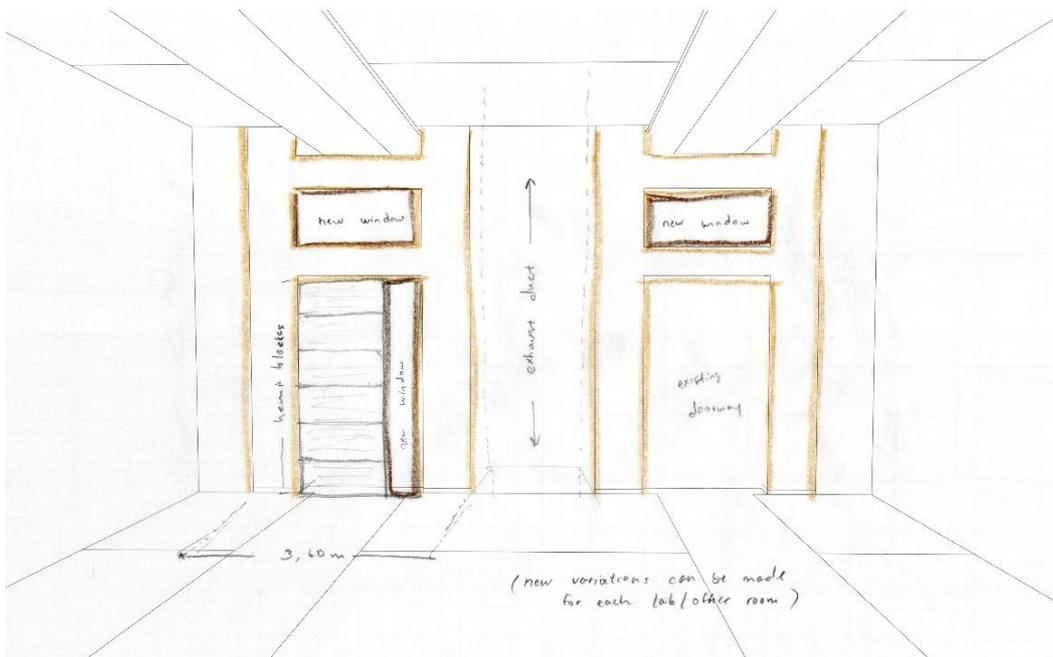
Appendix S : Impressions of a laboratory renovation strategy in the Kruytgebouw. Yellow is used to indicate the main 'H' and 'T' pre-fabricated concrete elements which are part of the remaining concrete structure.
