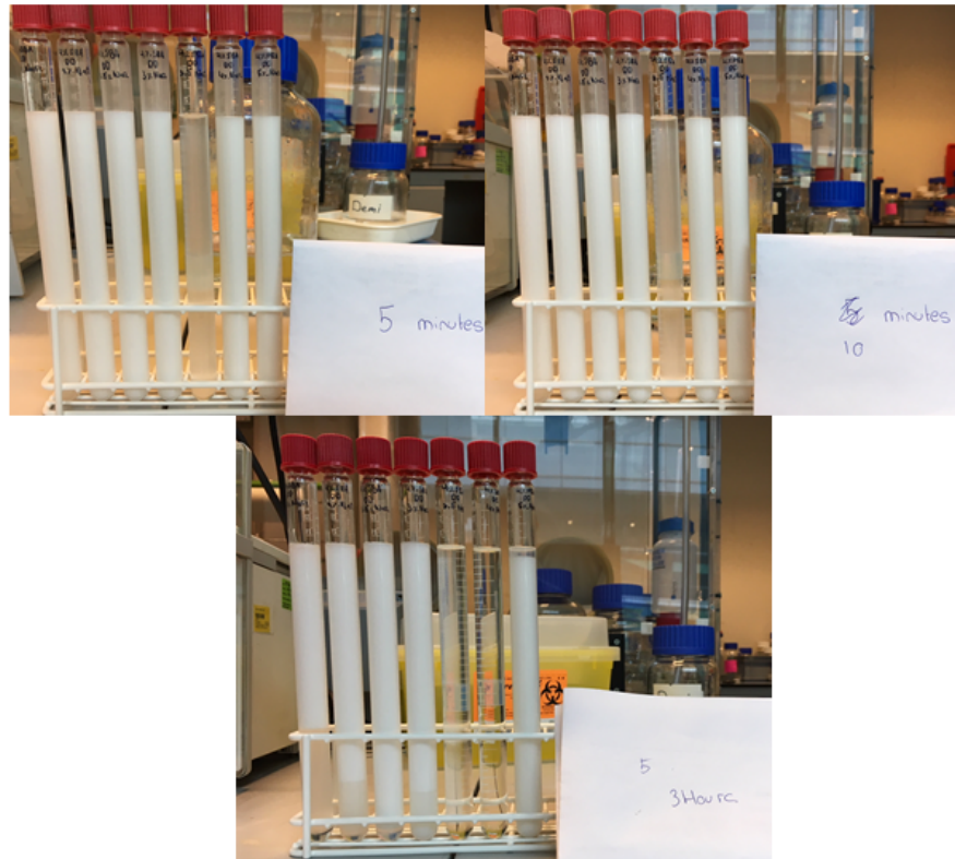
FIGURE A.2: Equilibration of the dodecane phase behaviour test. The tubes were agitated for 60 seconds and then left to settle. Photos were taken every 5 minutes initially and every hour afterwards.
