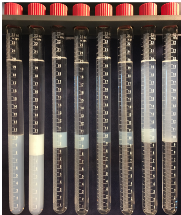
FIGURE 4.1: Phase behaviour of the dodecane-oil system using 1% O242 surfactant and 4% SBA as co-solvent. Salinities of the tubes are 2,3,3.25,3.5,3.75,4,5, respectively.
