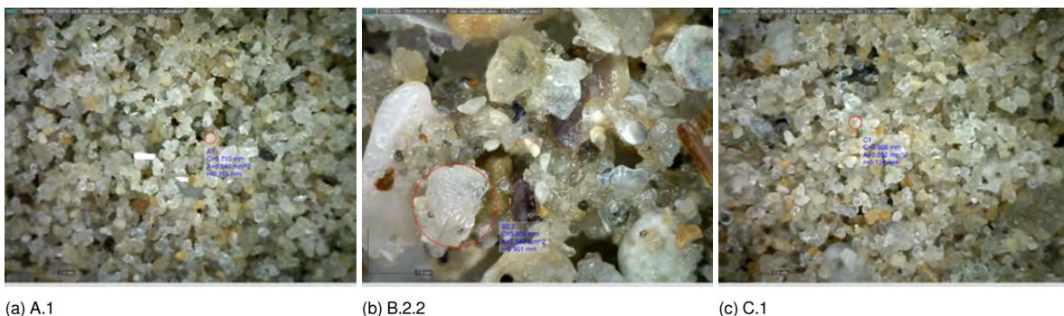
Figure D.18: Snapshots of some  $d_{50}$  measurements done for different samples with the Dino-Lite microscope
