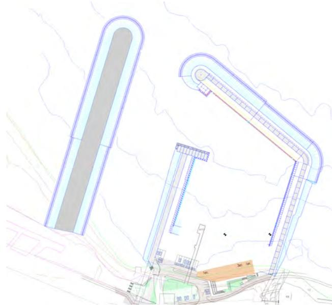
Figure 5.3: Blocking sediment using a groyne
