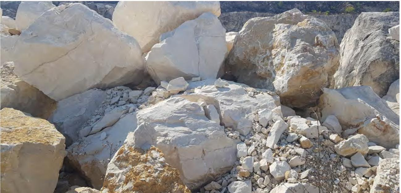
Figure E.18: Examples of damages of the large rocks in the pile
