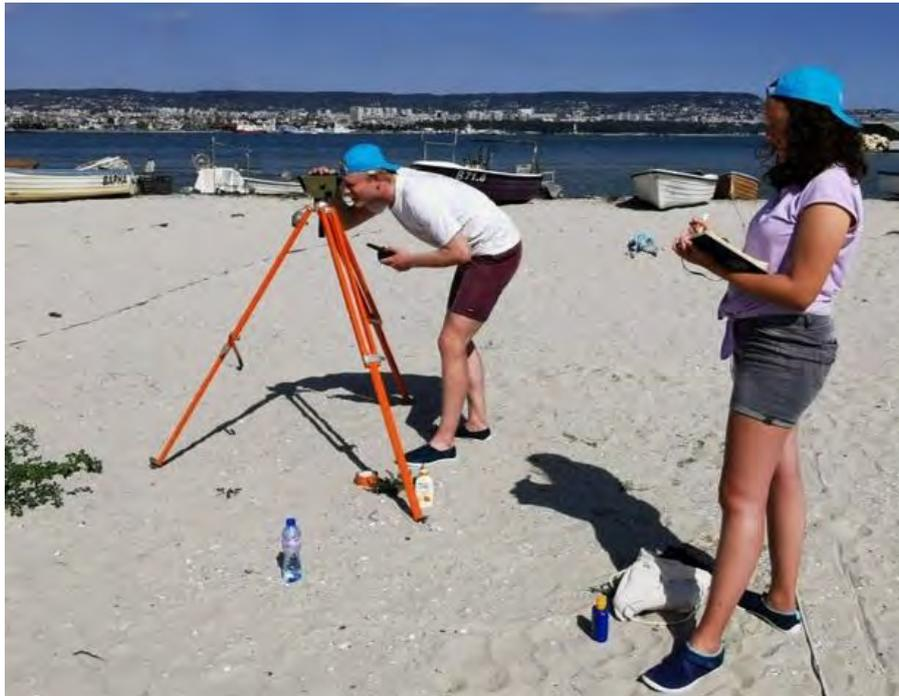
Figure D.5: Reading heights on levelling device standing on tripod
