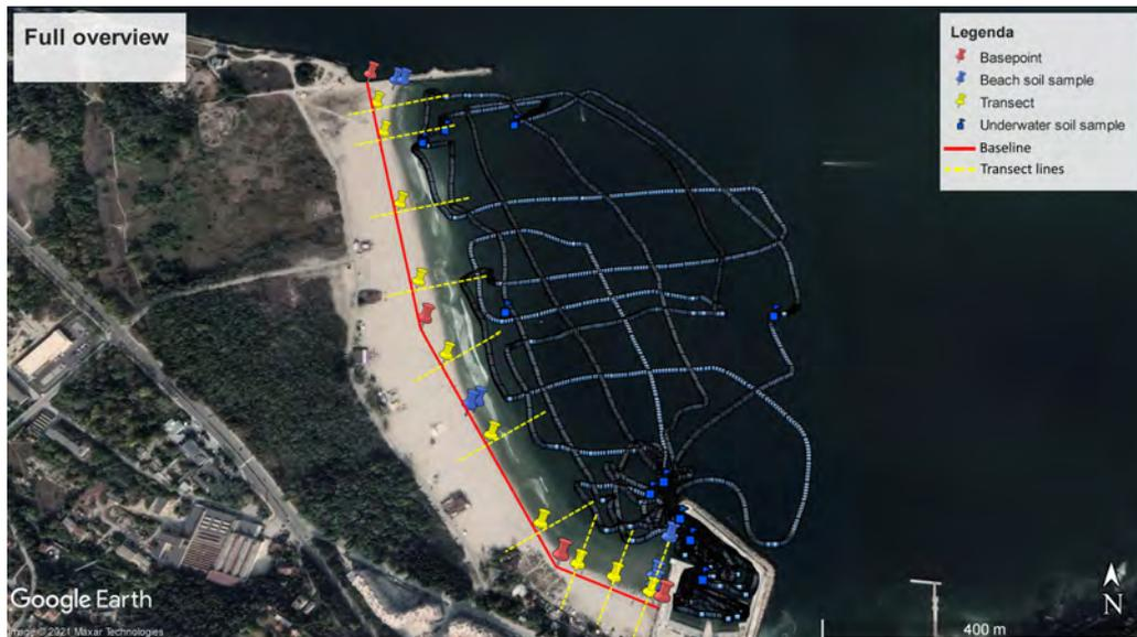
Figure D.10: Retrieved bathymetry depth samples
