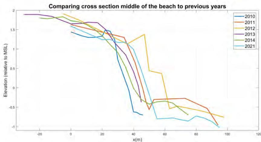
Figure E.3: Comparing cross section CD1 to similar cross section measurements from previous years
