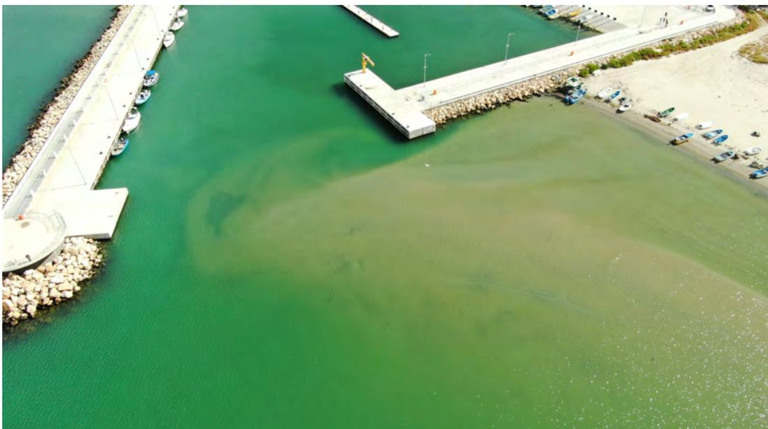
Figure 2.12: Karantinata Port entrance with excessive sedimentation
