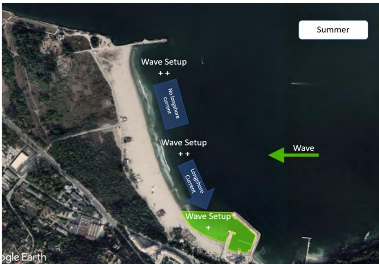
Figure 3.2: Wave Set-up and Longshore Current on Asparuhovo beach
