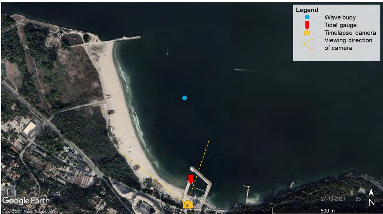
Figure 4.1: Locations of continuous measurement devices
