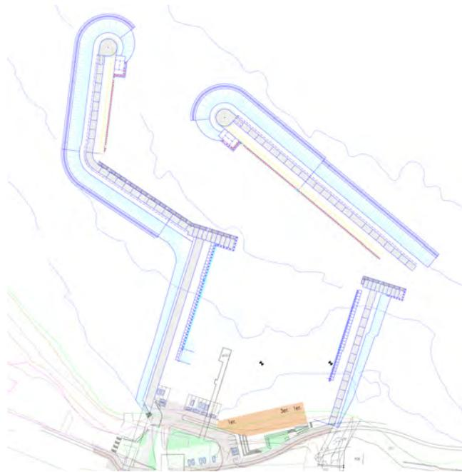
Figure 5.2: Relocation of the port entrance in combination with opening to change water flow
