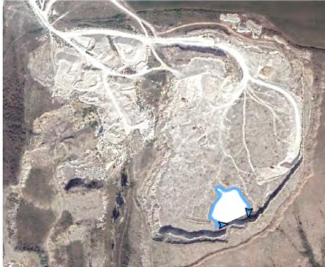
Figure D.13: GPS area measurement of big rock pile at Martsiana quarry
