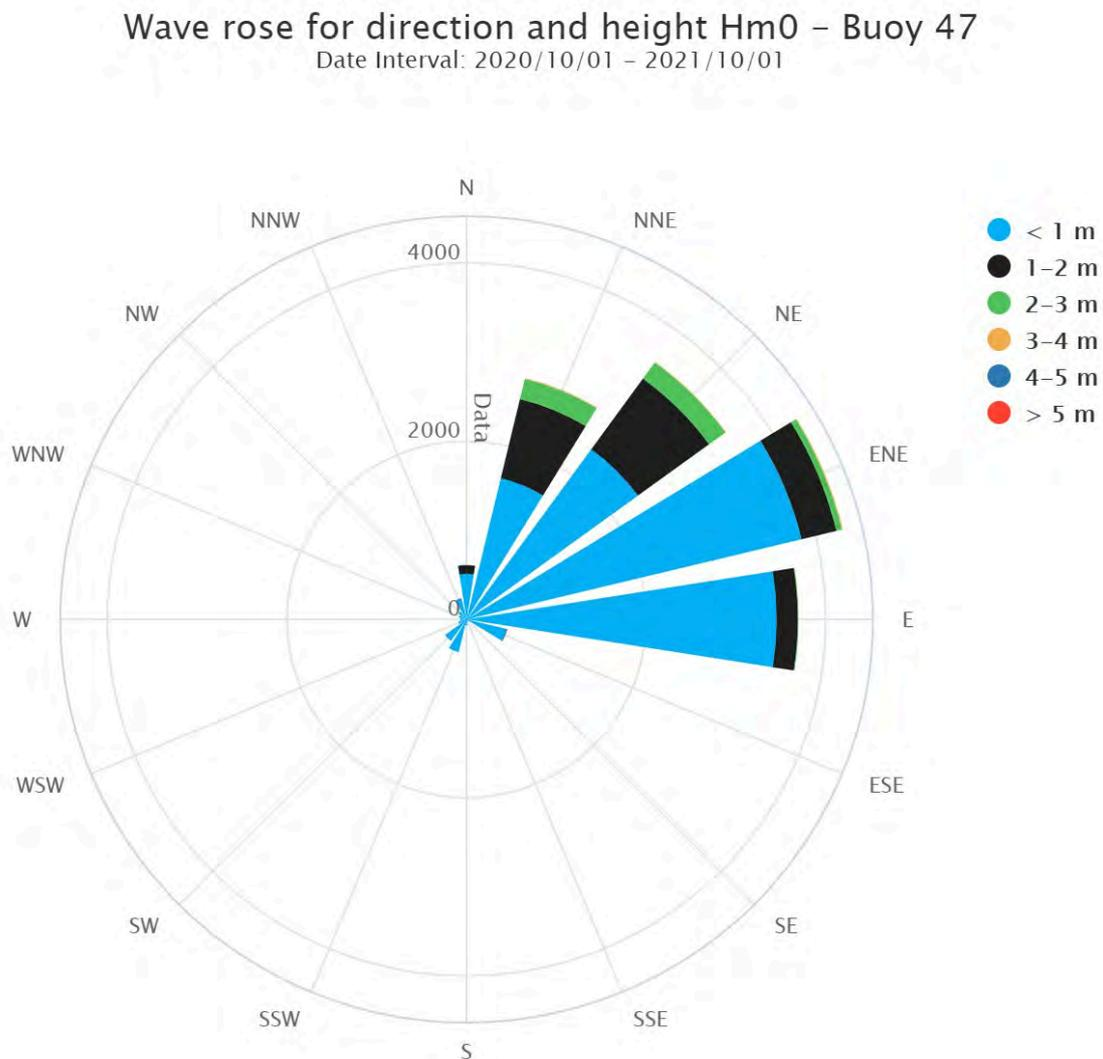
Figure E.6: Wave rose significant wave height for 1 year
