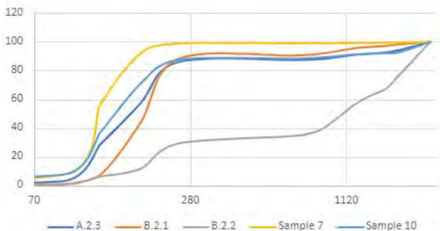
Figure E.5: Grain size distribution for samples A.2.3, B.2.1, B.2.2, Sample7 and Sample10
