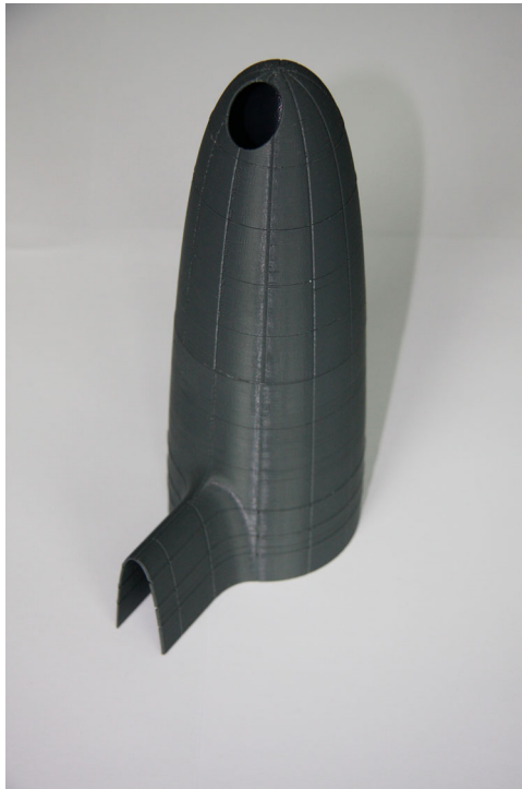
Figure 33. 3D printed thermoplastic model of the initial 1:500 scale hyperbolic shell.
