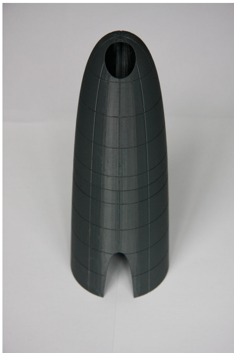
Figure 34. 3D printed thermoplastic model of the selected 1:500 scale hyperbolic shell, without entrance.
