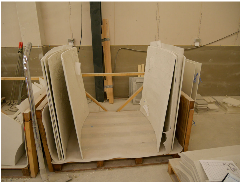
Figure 36. Finished cast panels for ring 1 and ring 2.
