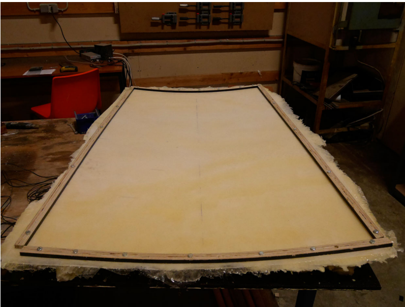
Figure 18. Fitting timber edges barriers on the mould.
