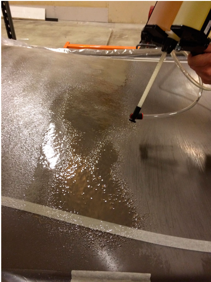
Figure 20. Applying the hard coat.
