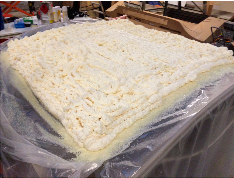
Figure 17. Curing the LDPU on the flexible table.
