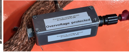
Figure 3.7: Measurements shunt(1000 ohm)
