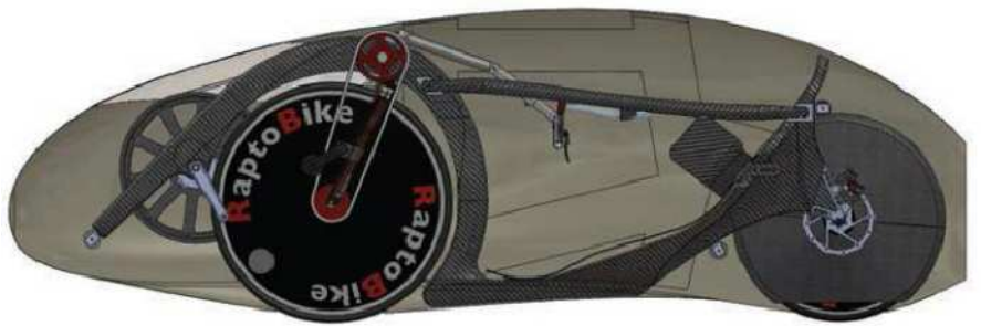
Figure 4. Design of the frame and all systems inside the fairing. Notice the two-stage driveline and the difference in size of the wheels.
