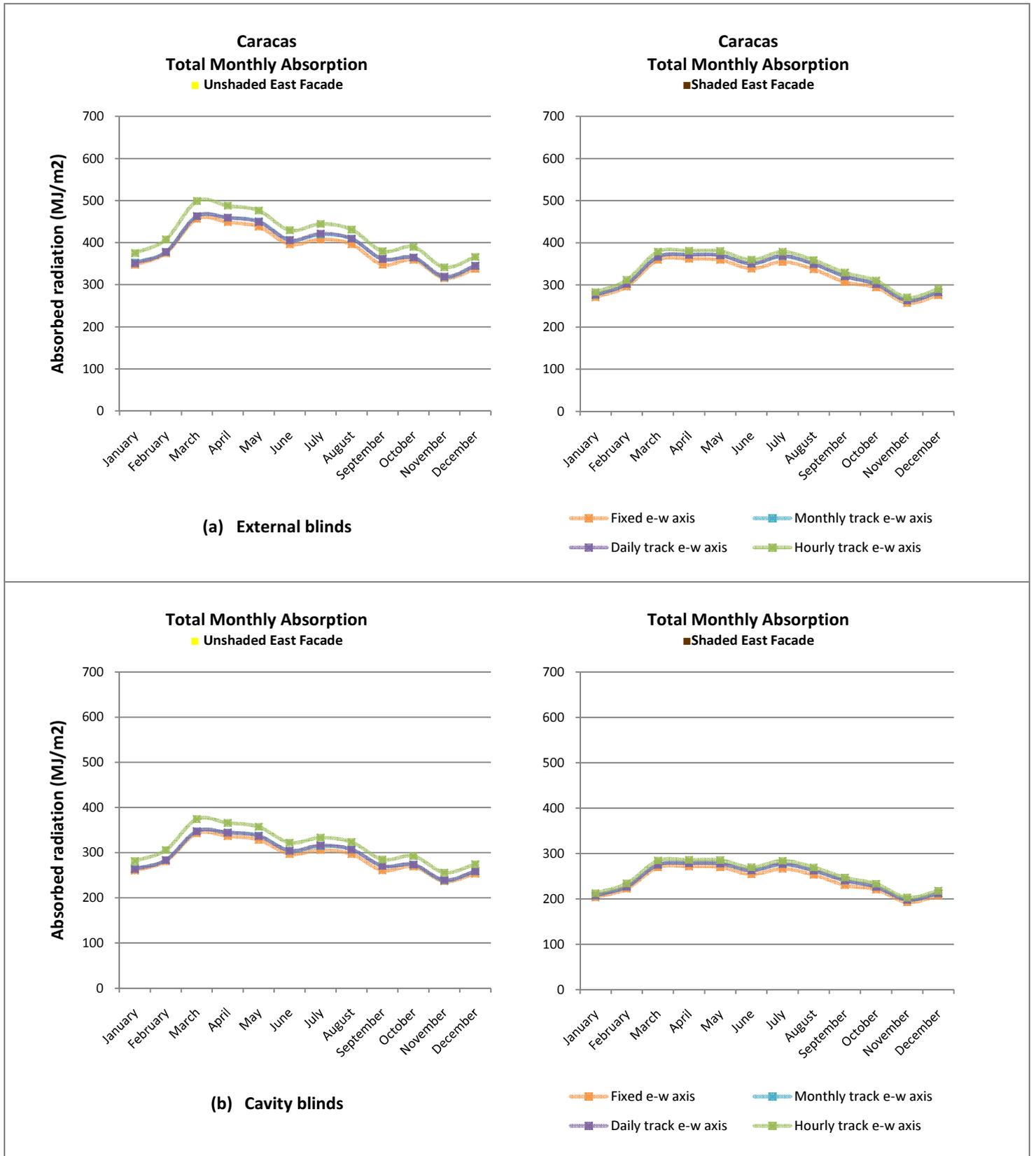
Figure 60. Absorption per m<sup>2</sup> of absorber surface for East and West Facade.
