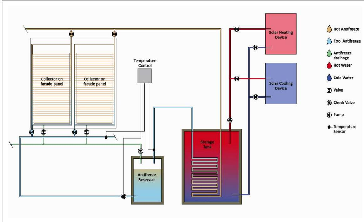
Figure 26. Solar thermal collection and cooling/heating systems interconnected.
