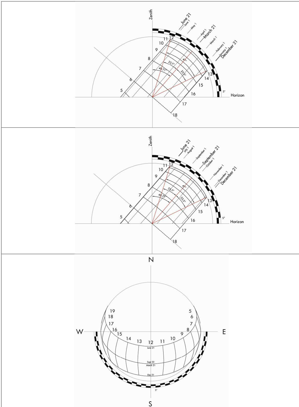
Figure 115. Sun path New York (40°43'N). Orthogonal projection.
