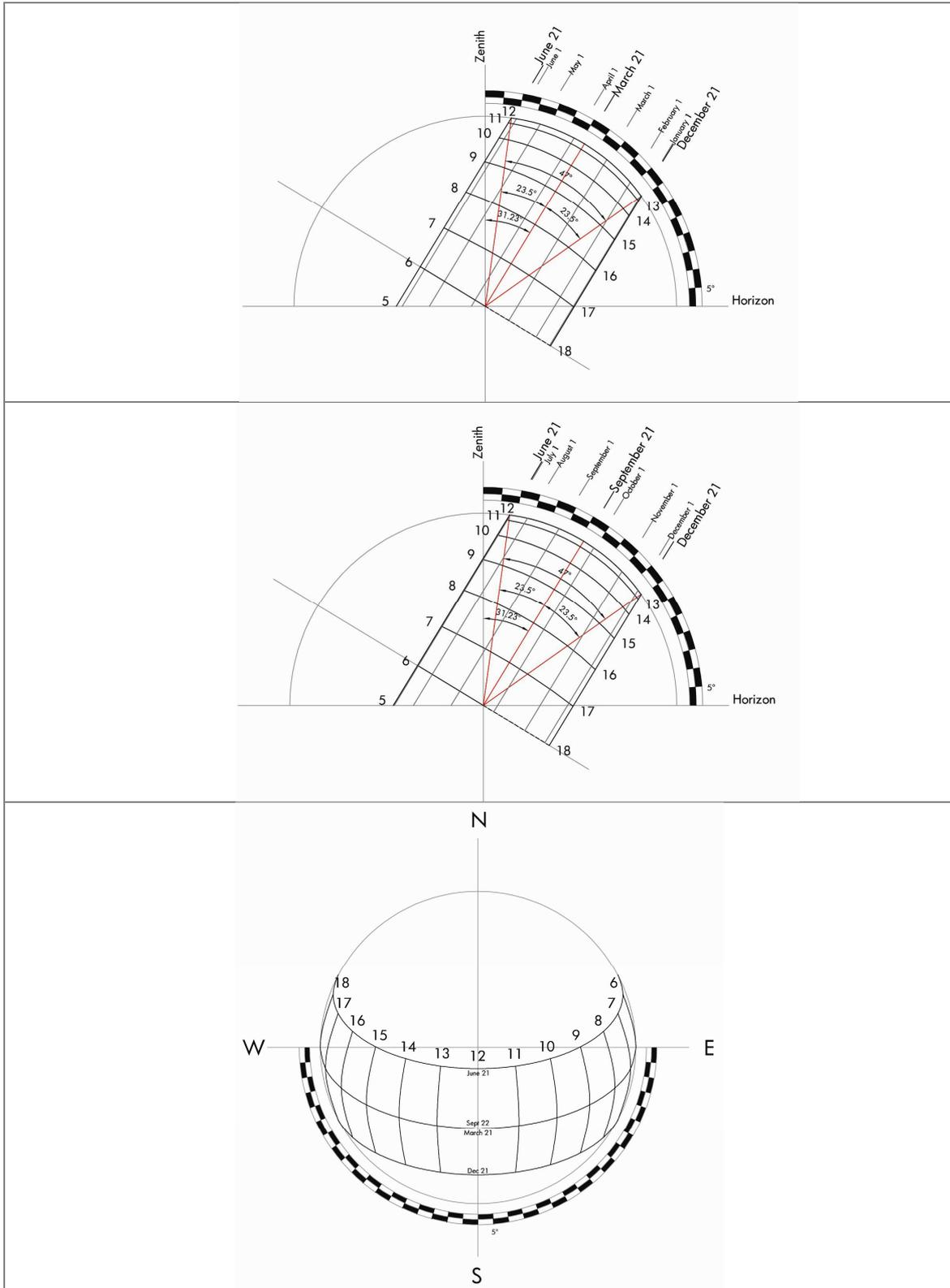
Figure 114. Sun path Shanghai (31°10'N). Orthogonal projection.
