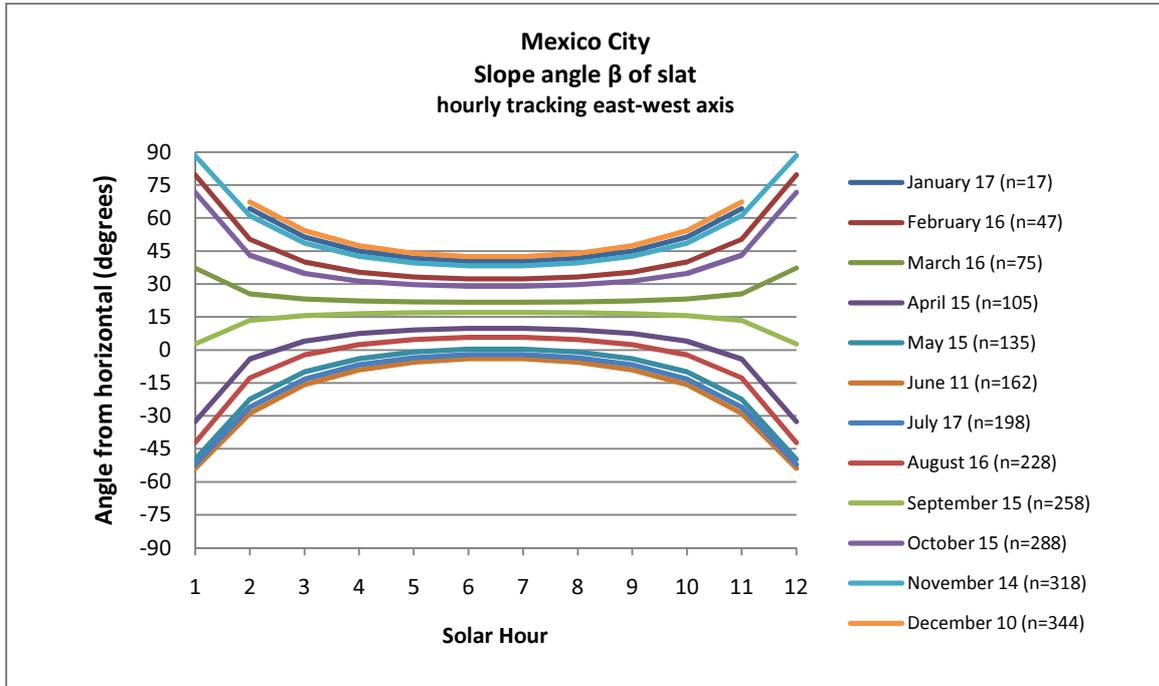
Figure 36. Slope angle for hourly angle adjustment for Mexico City.
