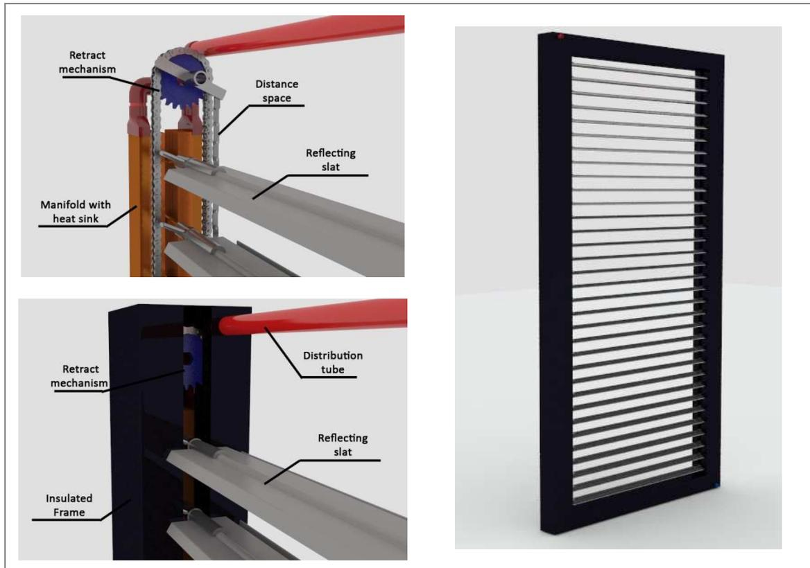
Figure 109. Fixed-angle retractable blind.
