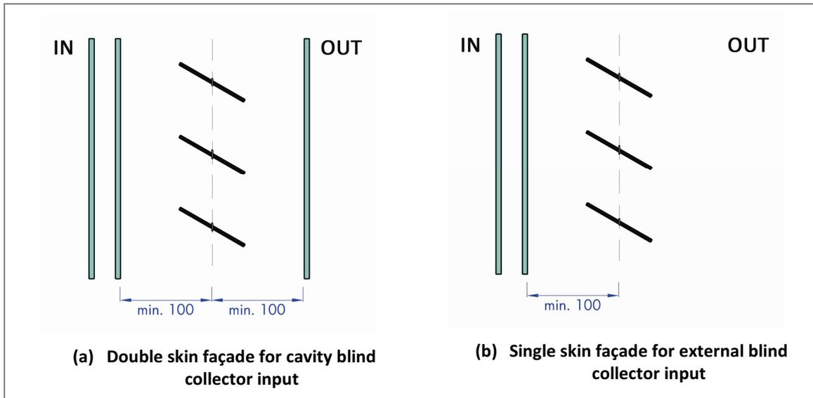
Figure 51. Façade layers for absorption and heat loss calculation.
