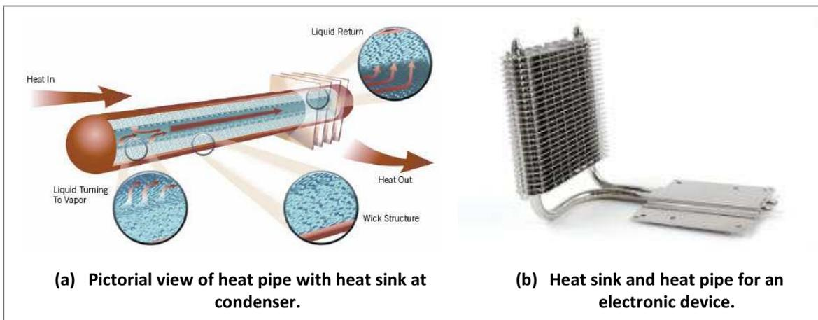
Figure 22. Heat pipe attached to heat sink. (Power Electronics Technology, 2011).
