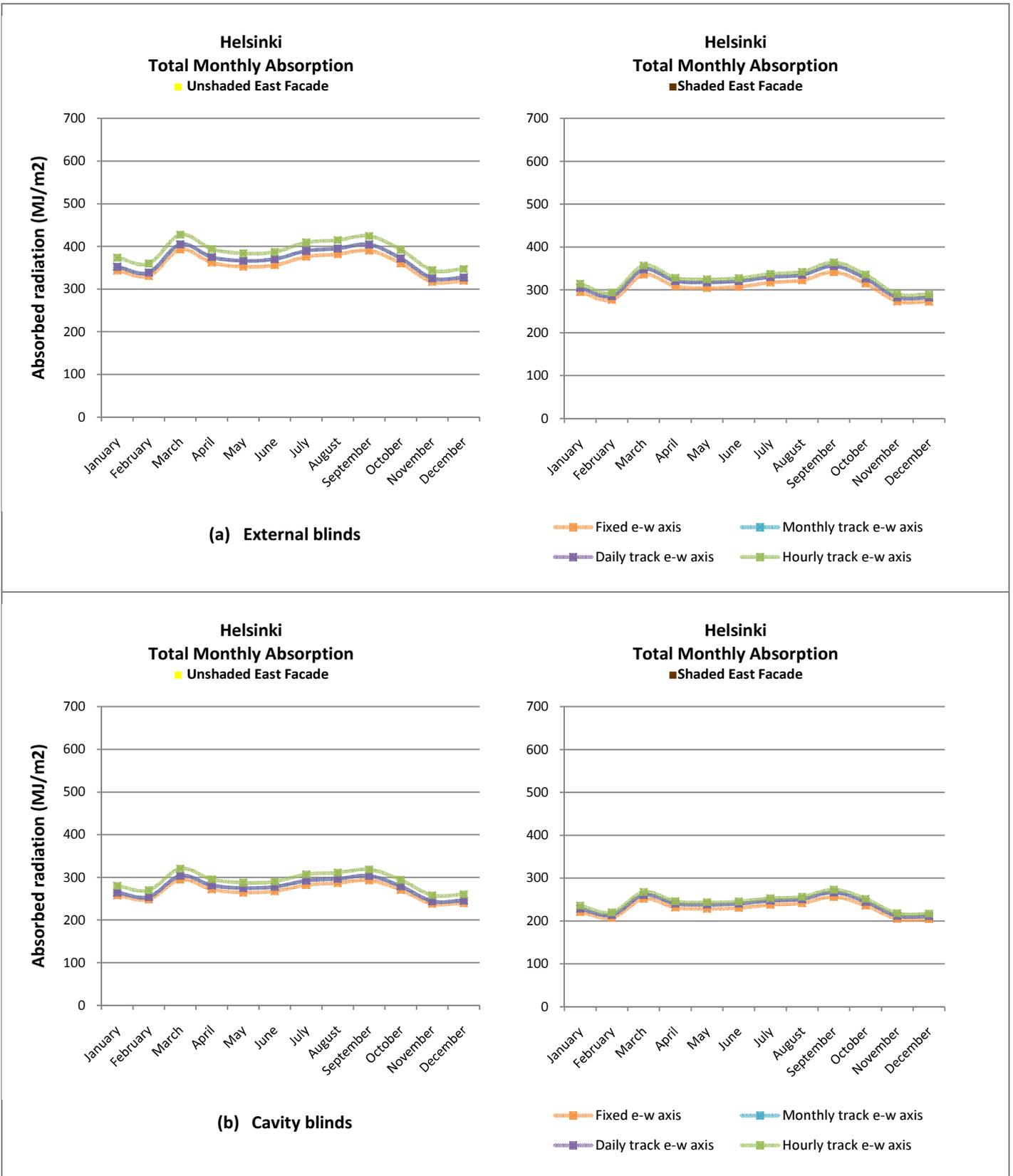
Figure 80. Absorption per m<sup>2</sup> of absorber surface for East and West Façade.
