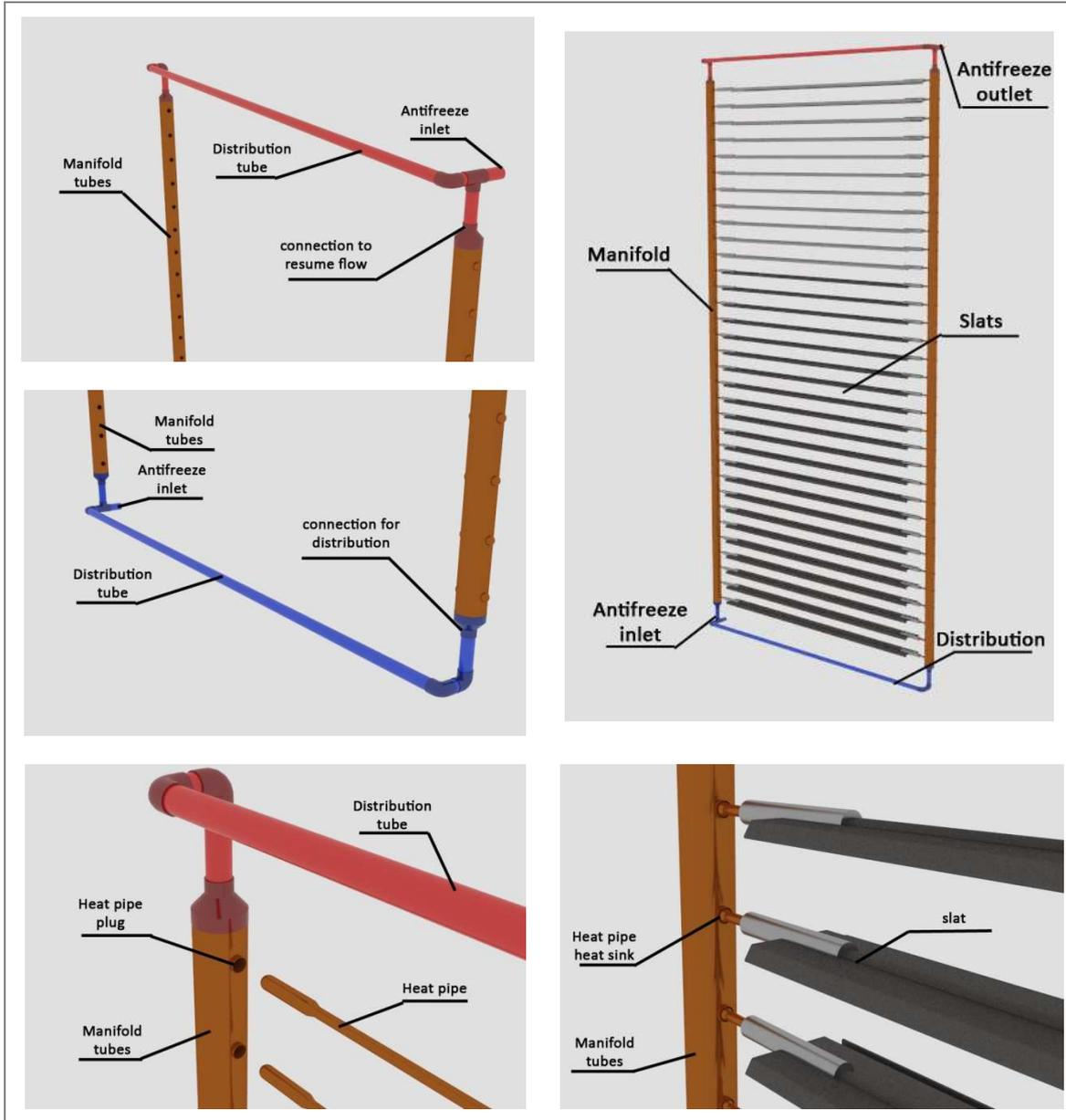
Figure 103. Manifold for fixed angle mechanism.
