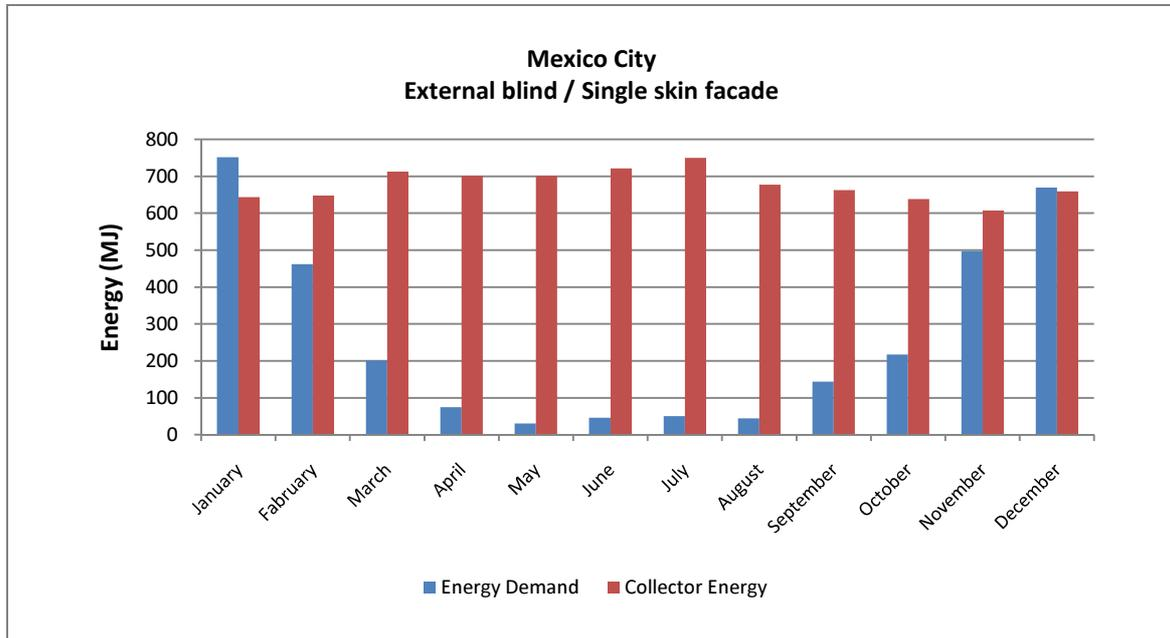
Figure 82. Energy demand and collector energy output for shaded external blinds.
