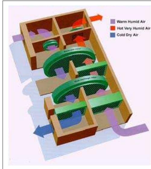
**Figure 15. Desiccant cooling system.**
