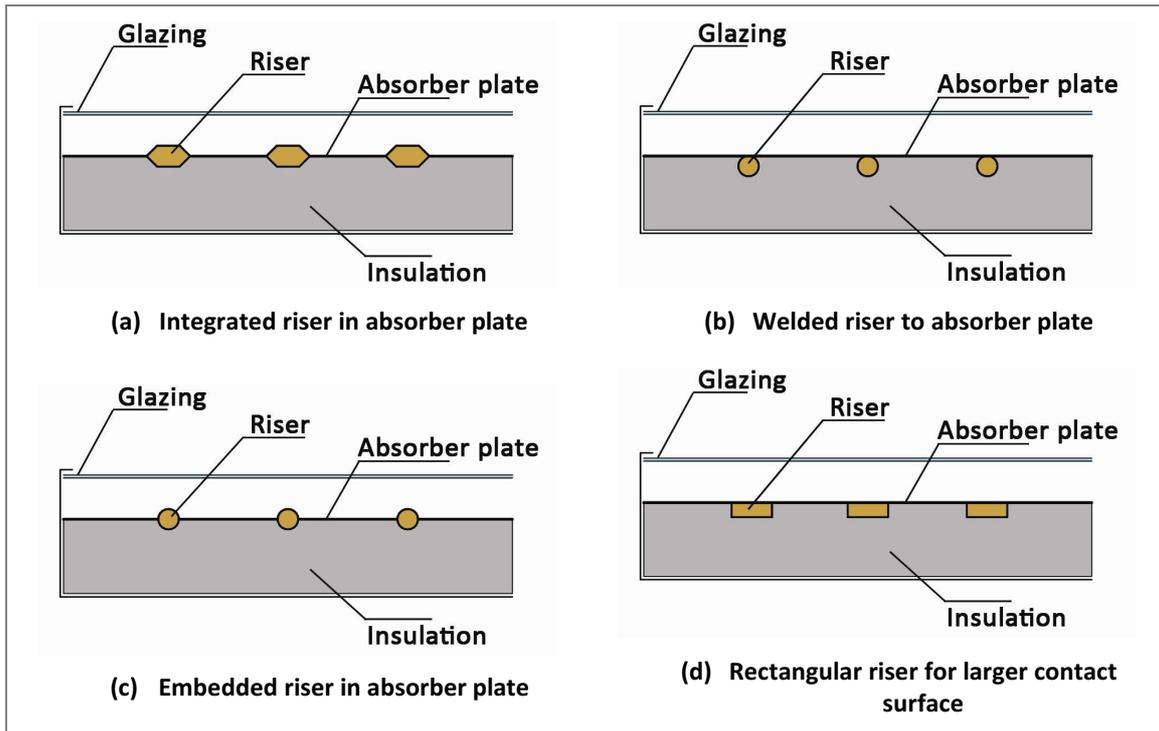
Figure 92. Various ways of bonding absorber and risers in a flat plate collector
