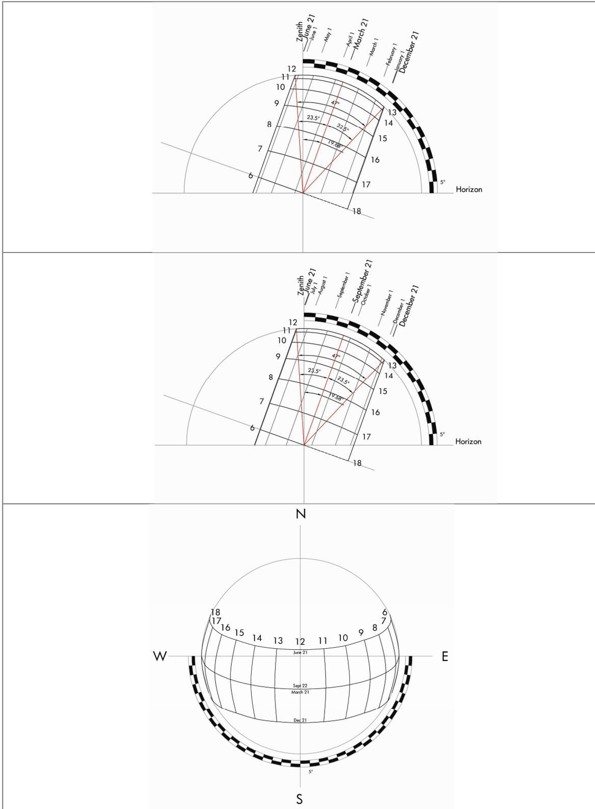
Figure 113. Sun path Mexico (19°41'N). Orthogonal projection.
