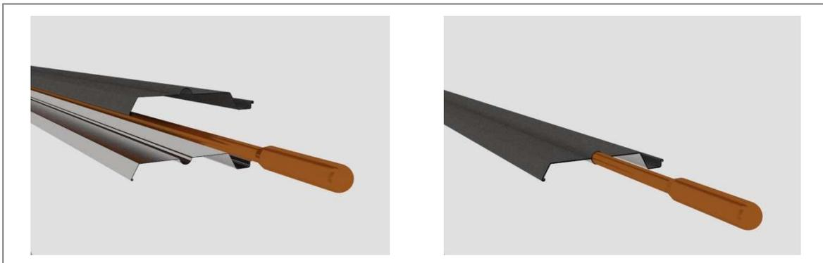
Figure 93. Slat and heat pipe connection.
