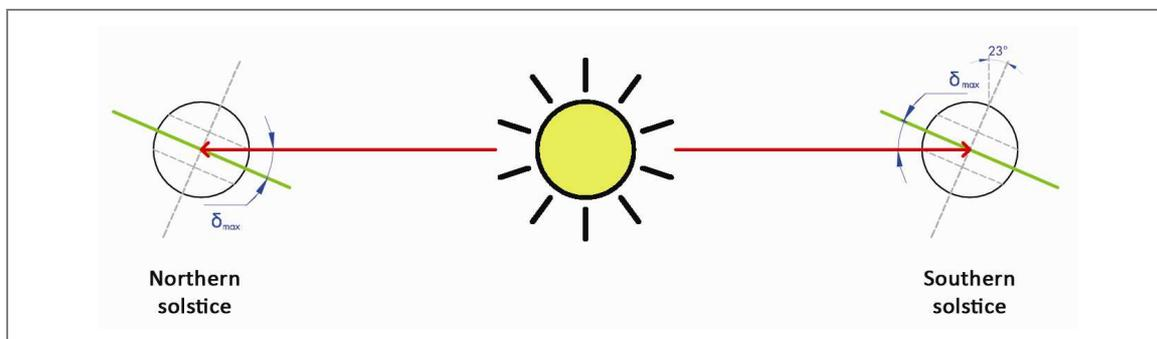
**Figure 31. Declination angle of the rays of the sun and the earth's Equator.**
