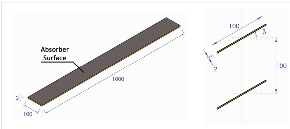
Figure 49. Slat geometry parameters for calculations input.
