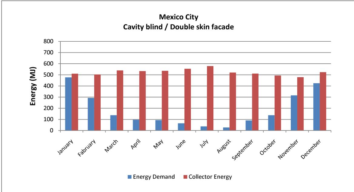
Figure 83. Energy demand and collector energy output for shaded cavity blinds.
