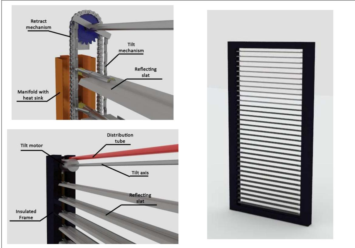
Figure 110. Tiltable and retractable blind
