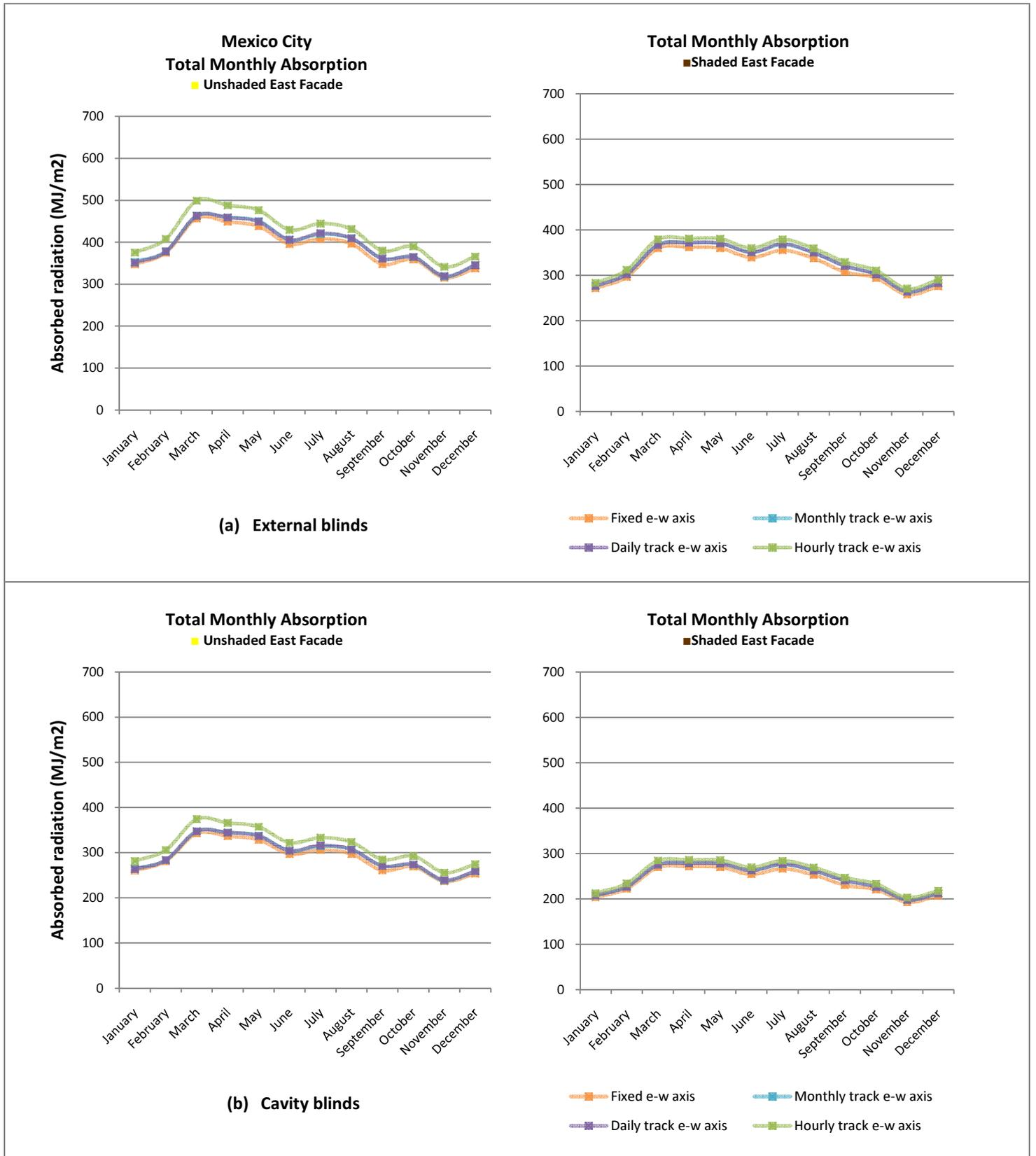
Figure 64. Absorption per m<sup>2</sup> of absorber surface for East and West Façade.
