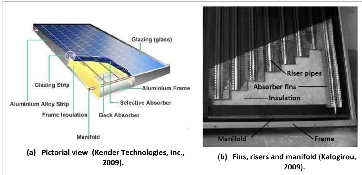
Figure 11. Typical flat-plate collector
