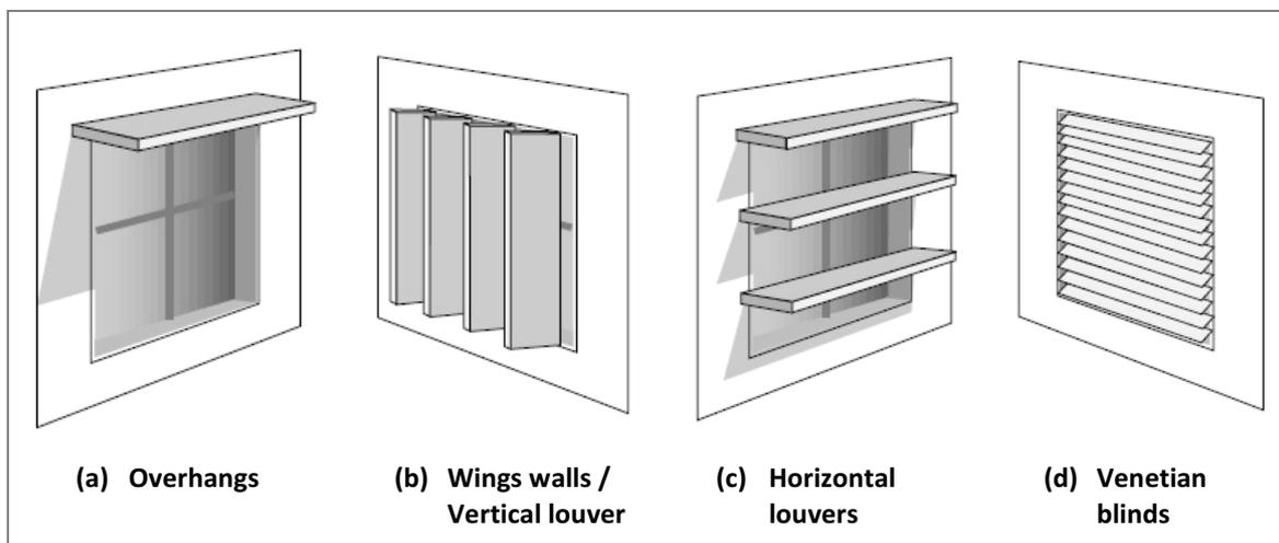
Figure 5. Different sun shading systems .
