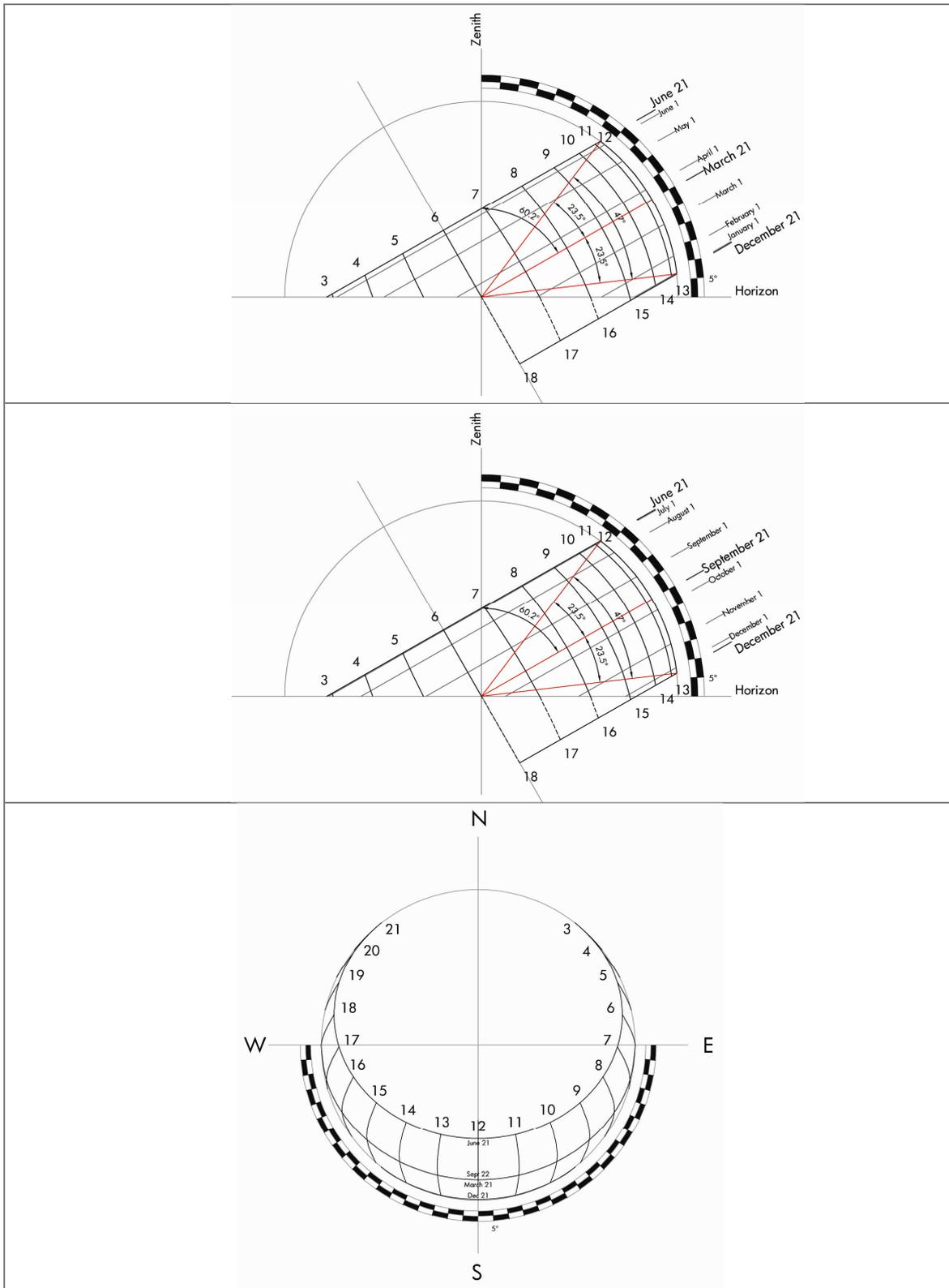
Figure 117. Sun path Helsinki (60°12'N). Orthogonal projection.
