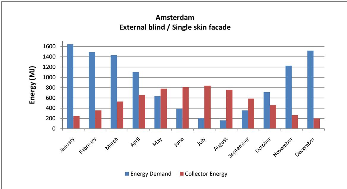
Figure 84. Energy demand and collector energy output for shaded cavity blinds.
