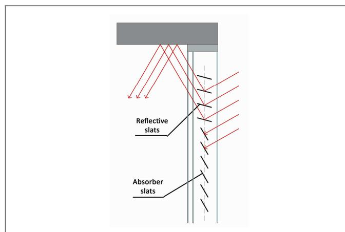
Figure 86. Different angle in upper slats for light income.
