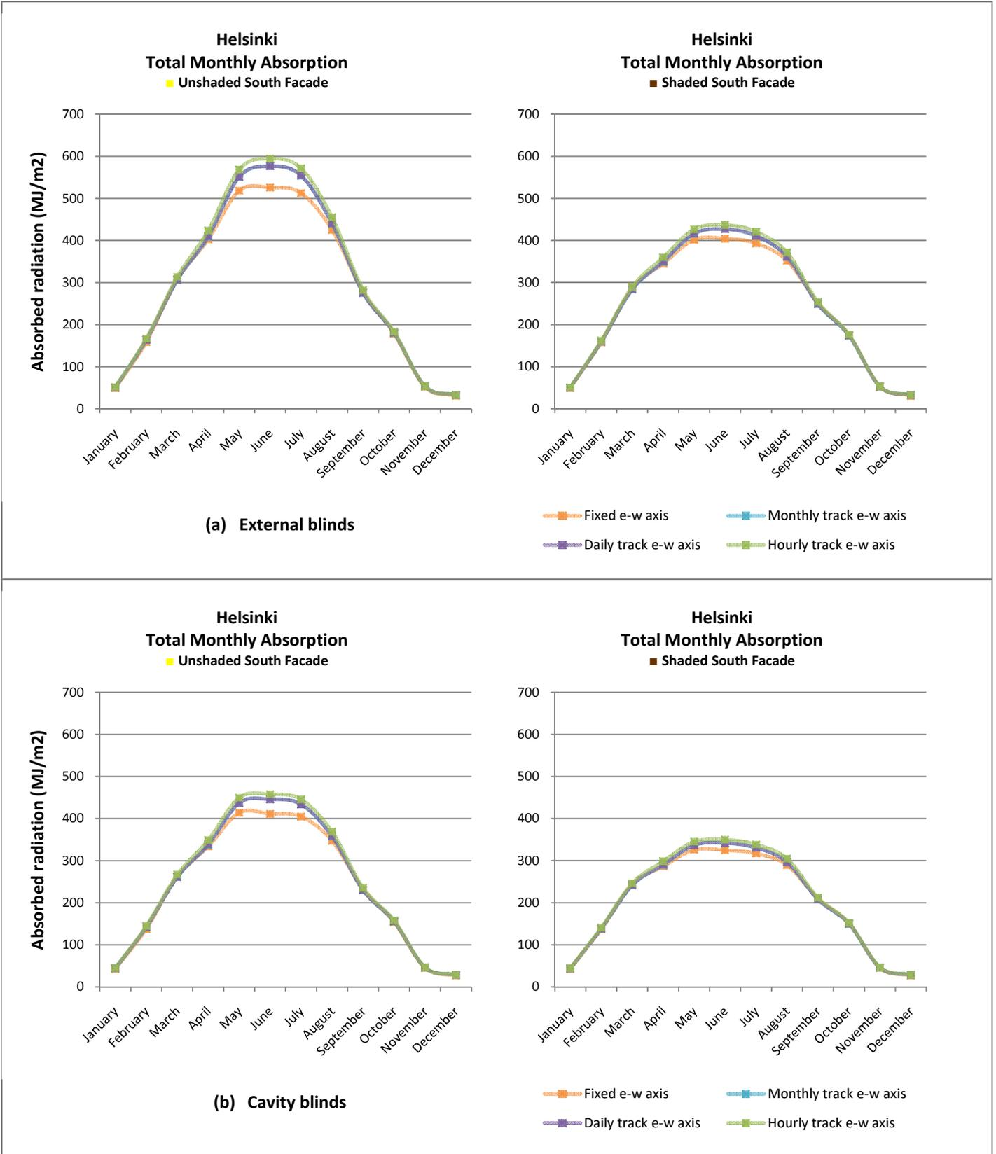
Figure 78. Absorption per m<sup>2</sup> of absorber surface for South Façade.
