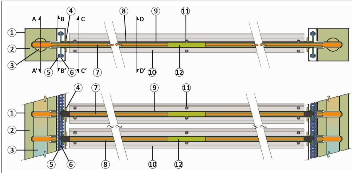
**Figure 119. Top and front view of the mechanism for a blind that tilts.**
