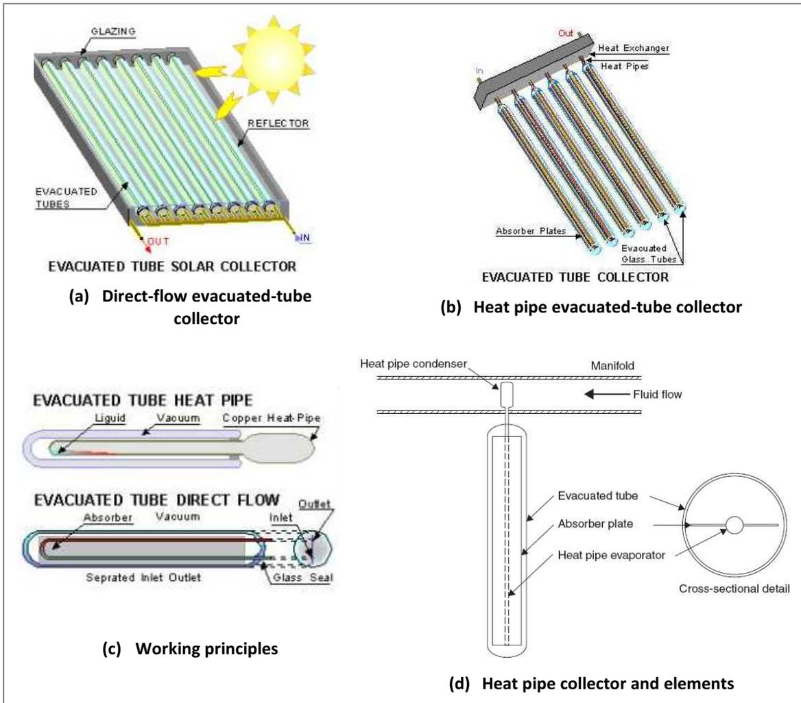
Figure 12. Evacuated-tube collectors and their elements (Encyclopedia of Alternative Energy and Sustainable Living, 2010).
