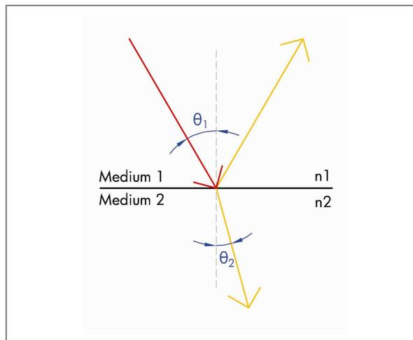
**Figure 47. Incident and refraction angles for a ray that passes through different media.**
