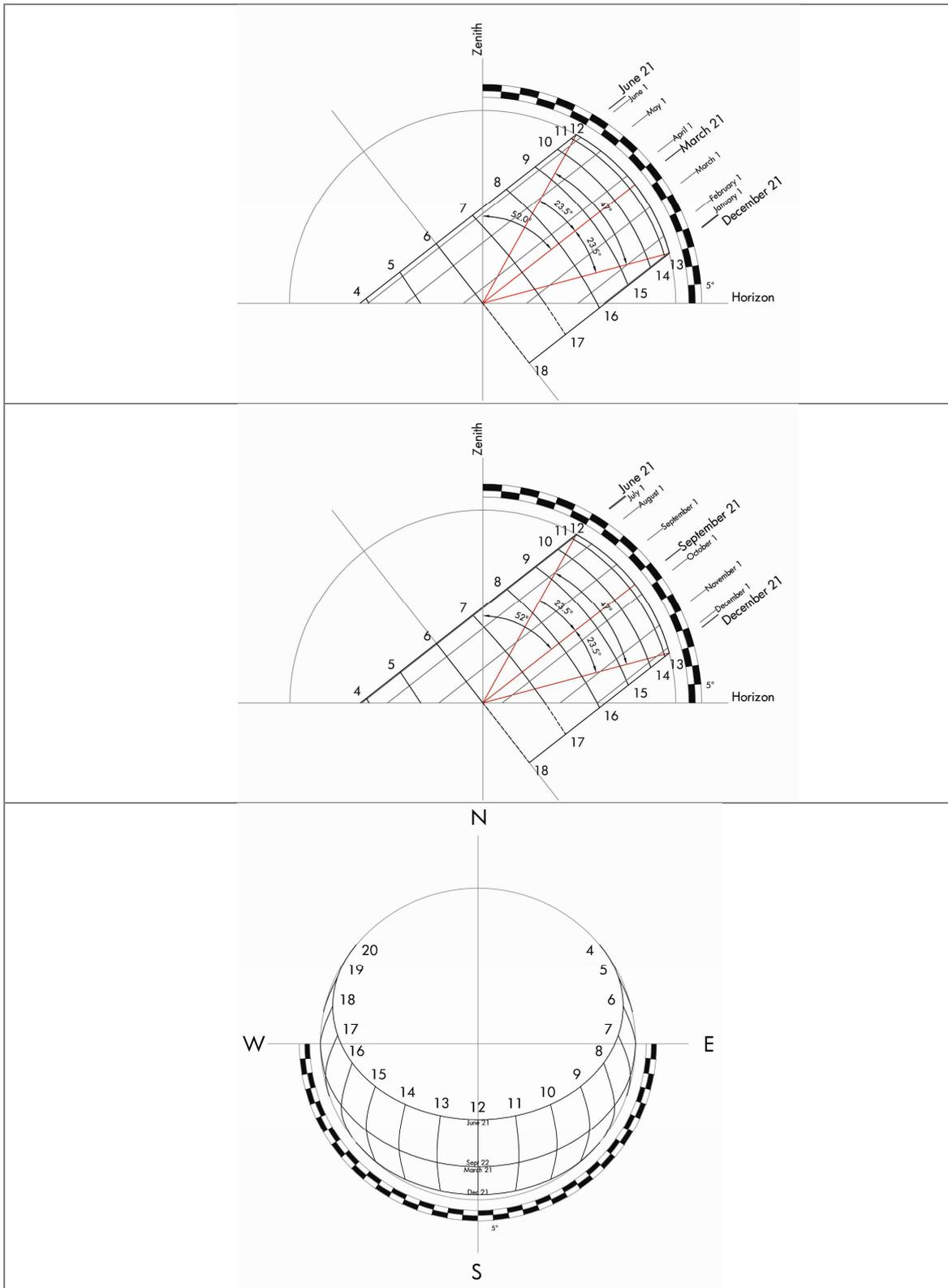
Figure 116. Sun path Amsterdam (52°22'N). Orthogonal projection.
