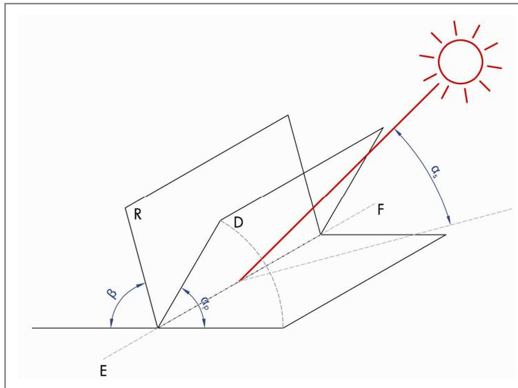
Figure 39. The solar altitude angle  $\alpha_s$ , and the profile angle  $\alpha_p$ , for surface R
