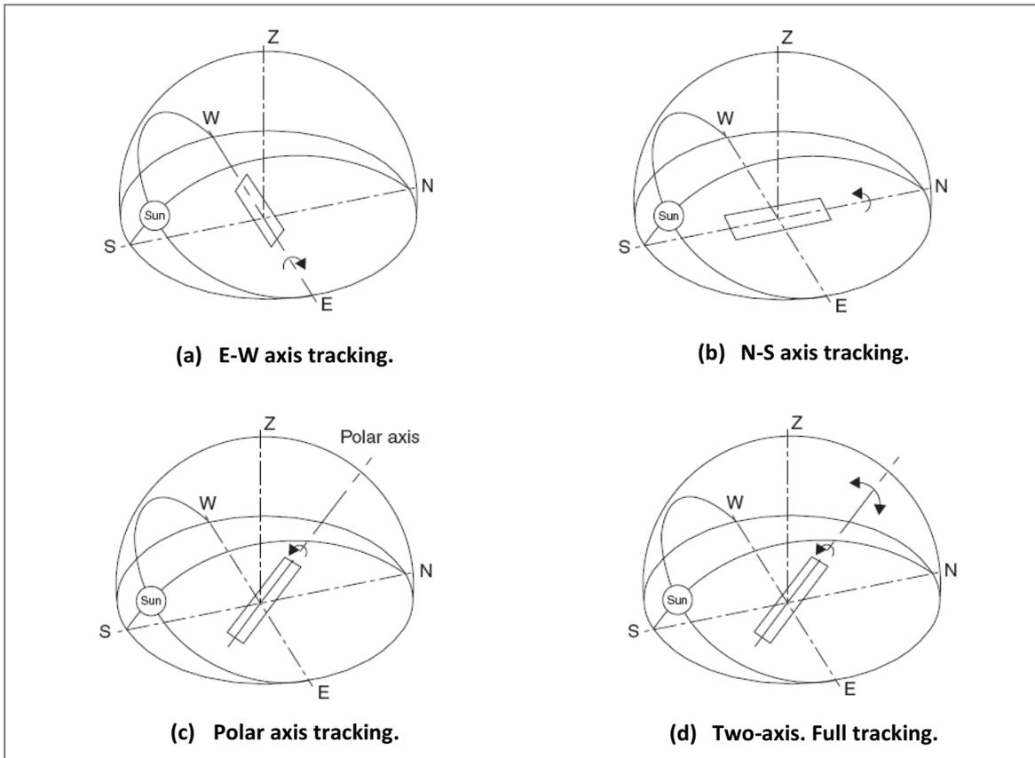
Figure 34. Various models of solar tracking (Kalogirou, 2009).
