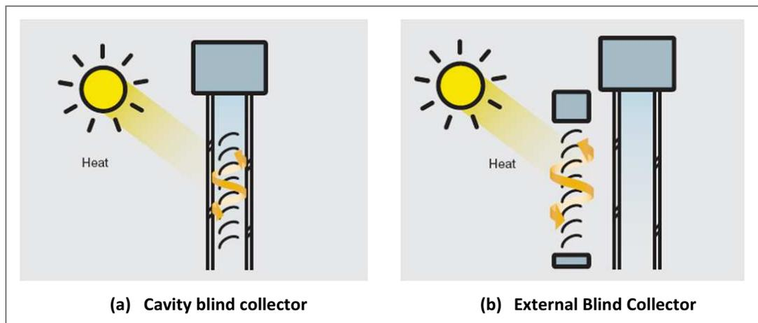
Figure 24. Blind collector placed inside the cavity and in front of the façade (Zumbotel, 2010).
