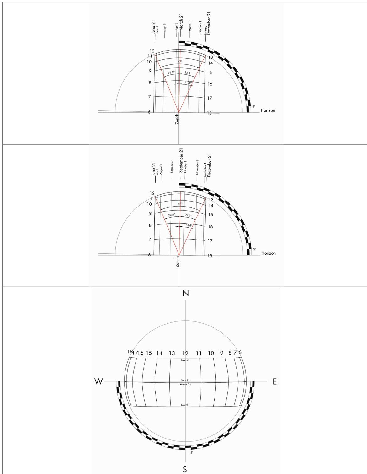
Figure 111. Sun path Singapore (1°17' N). Orthogonal projection.
