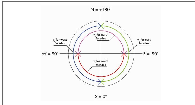
**Figure 46. Incidence of radiation in façades.**
