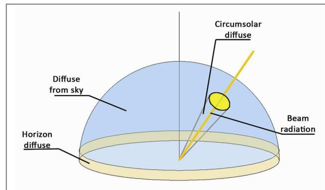
**Figure 38. Distribution of diffuse radiation over the sky dome.**
