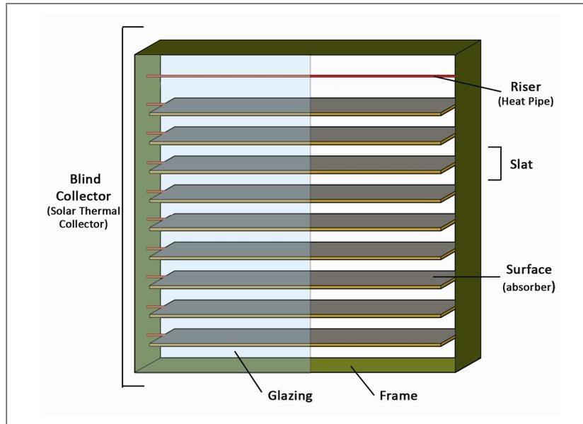
Figure 23. Parts of a Venetian Blind Solar Thermal Collector.
