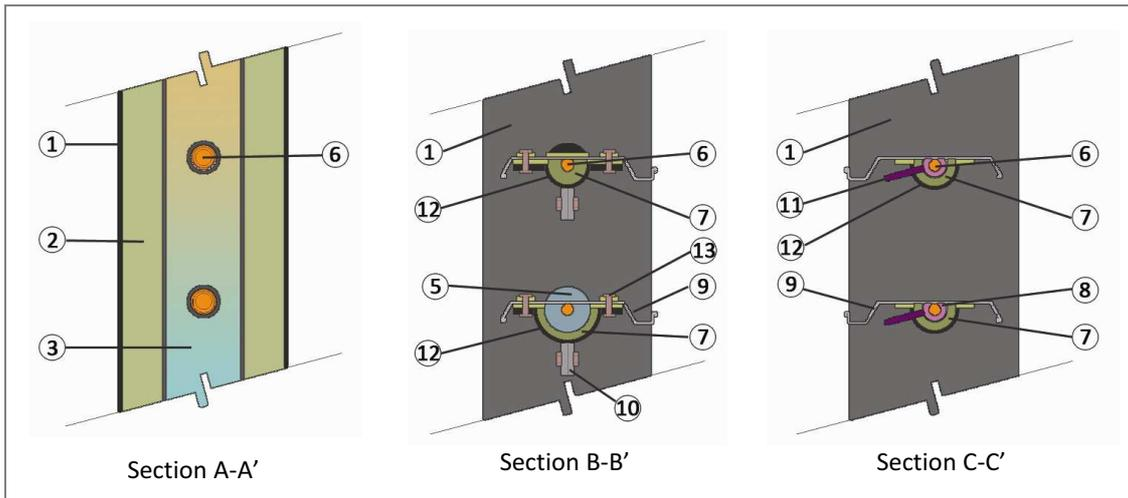
**Figure 107. Section A-A': Manifold with heat pipe heads embedded. Section B-B': Two different gripping mechanisms. Section C-C': Spring and lever.**
