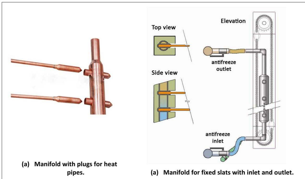
Figure 102. Principle of manifold for non-retractable blinds.
