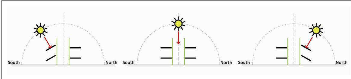
Figure 37. Slope angle  $\beta$  of slats when no solar radiation is falling on a particular façade.
