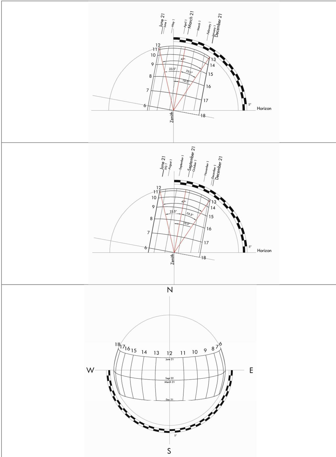
Figure 112. Sun path Caracas (10°30'N). Orthogonal projection.
