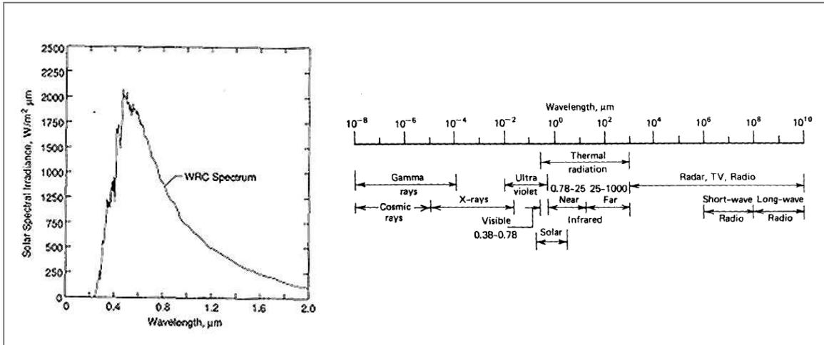
Figure 4. The WRC standard spectral irradiance curve at mean earth-sun distance (Duffie, 2006).
