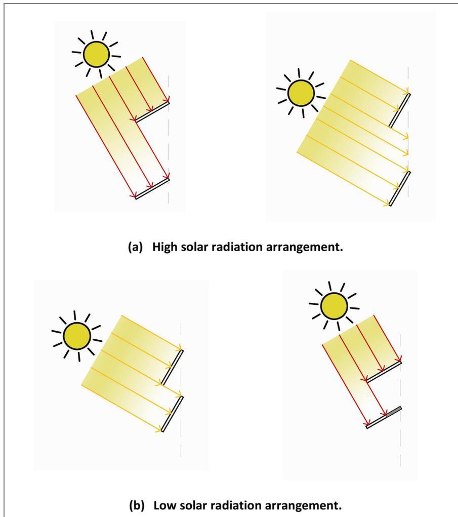
Figure 43. Offset of slats according to solar elevation.
