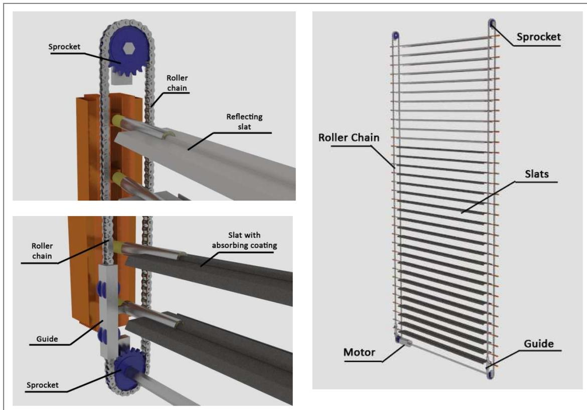
Figure 98. Retracting Mechanism.
