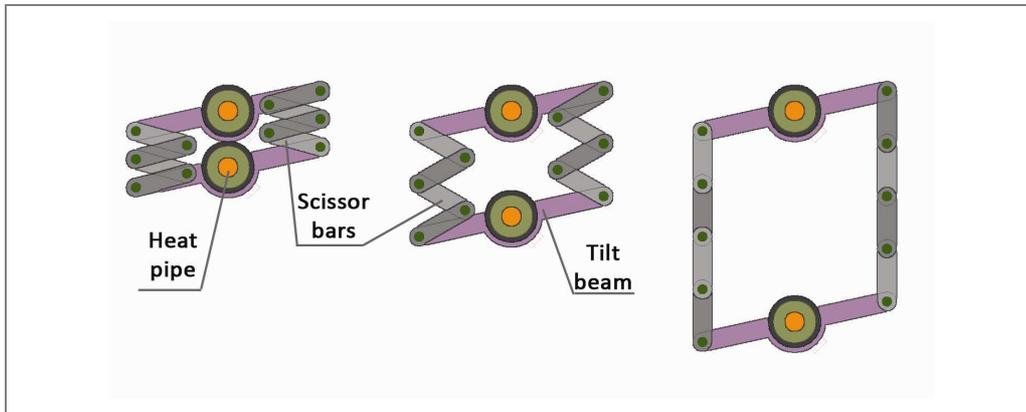
Figure 100. Scissor-like chain for tilting.
