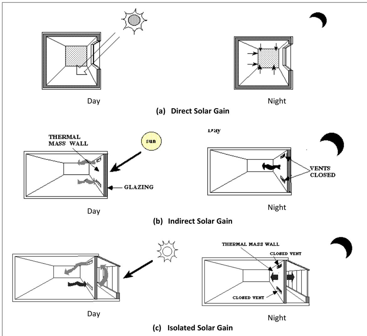
Figure 8. Passive solar heating systems (Passive Solar Design, 2010).
