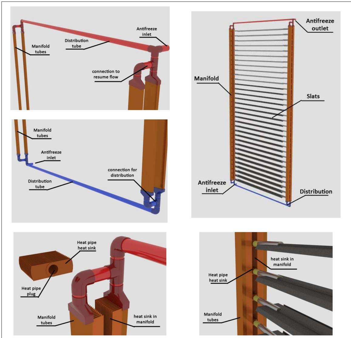
Figure 105. Manifold for retractable mechanism.
