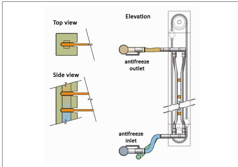
**Figure 104. Manifold for retractable blinds. Two flatten tubes run next to the heat pipe heads along the length of the frame.**
