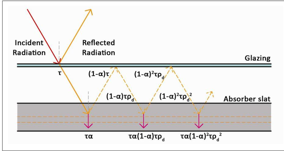
Figure 48. Top view of façade showing radiation transfer between glazing and absorber slats.
