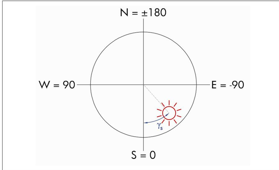
Figure 33. Solar Azimuth Angle  $\gamma_s$  seen from top view.
