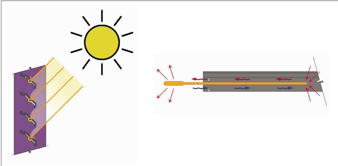
**Figure 25. First part of the system: Collection of solar thermal energy through slats in a venetian blind.**
