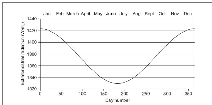
Figure 3. Variation of the extraterrestrial solar radiation throughout the year (Duffie, 2006).
