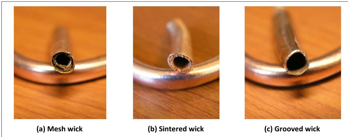
Figure 18. Different wick on heat pipes (Frosty Tech, 2010).
