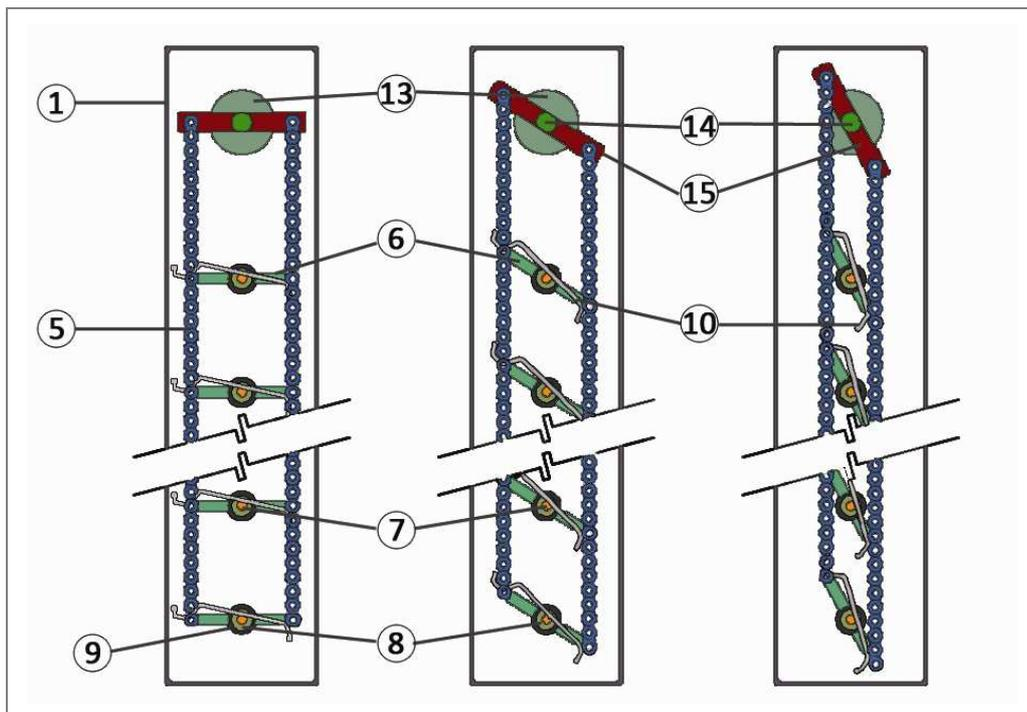
**Figure 118.** Tilting mechanism for tracking blind.
