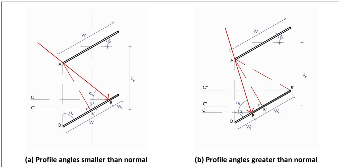
Figure 42. Geometry of shading on fixed slats.
