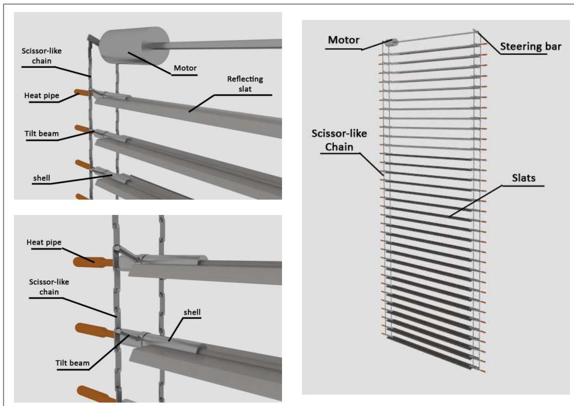
Figure 101. Tilt mechanism
