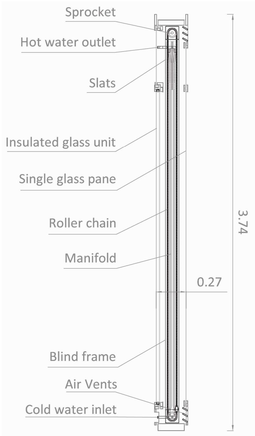
Plan 1. Vertical section of façade panel with solar thermal collector blind embedded.
