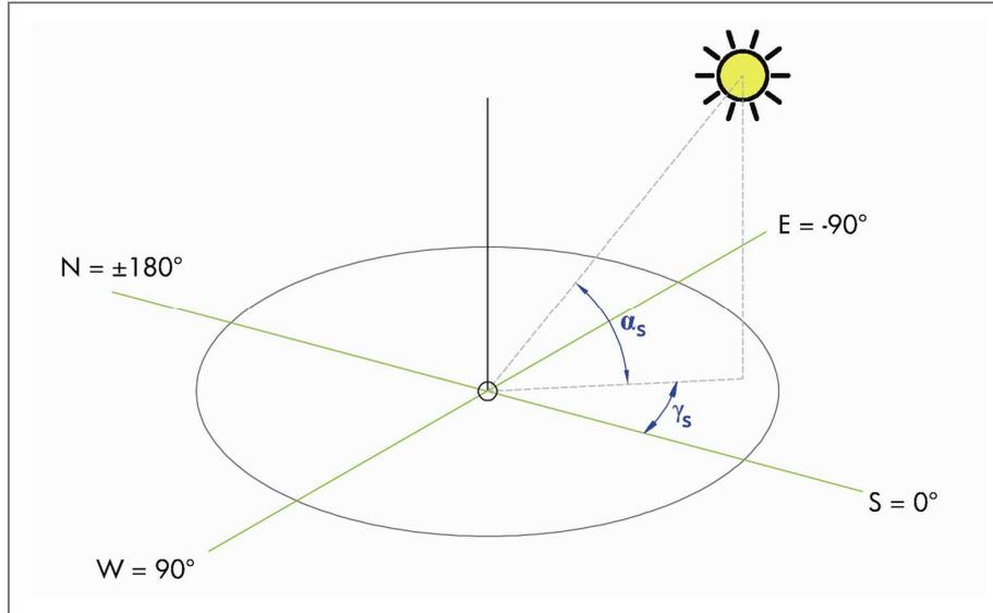
Figure 30. Solar altitude angle  $\alpha_s$  and Solar azimuth angle  $\gamma_s$ .
