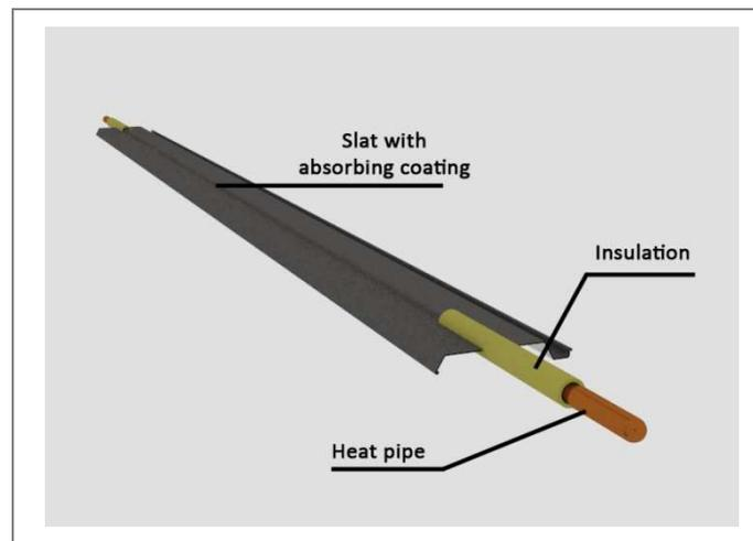
Figure 94. Insulation of heat pipe
