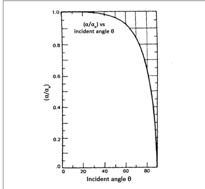
Figure 44. Ratio of solar absorptance to solar absorptance at normal incident for a flat black surface (Duffie, 2006).
