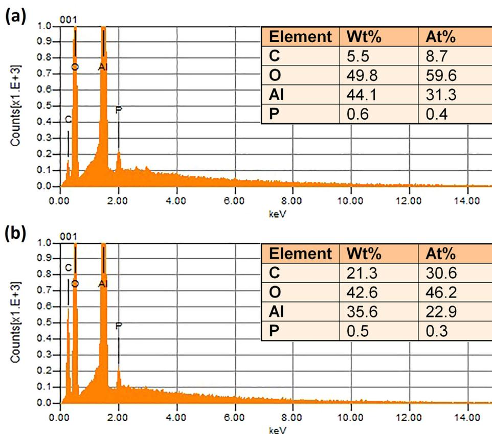
Fig. 3. Elemental analysis of the (a) unmodified and (b)  $\gamma$ -alumina-g-C<sub>10</sub> membrane by EDX.
