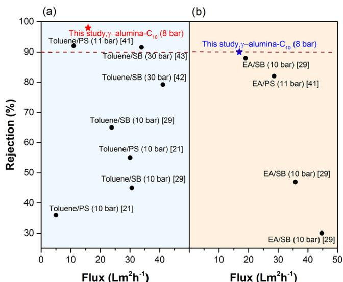
**Fig. 8.** Comparison of the OSN performance of  $\gamma$ -alumina-g-C<sub>10</sub> membrane with previously reported functionalized ceramic membranes [21,29,41] and commercially polymeric STARMEM 122 membrane [42,43]: (a) SB or polystyrene (PS,  $M_w$  580 Da)/toluene and (b) SB/EA were used as model feed. The dotted line represented 90% solute rejection.
