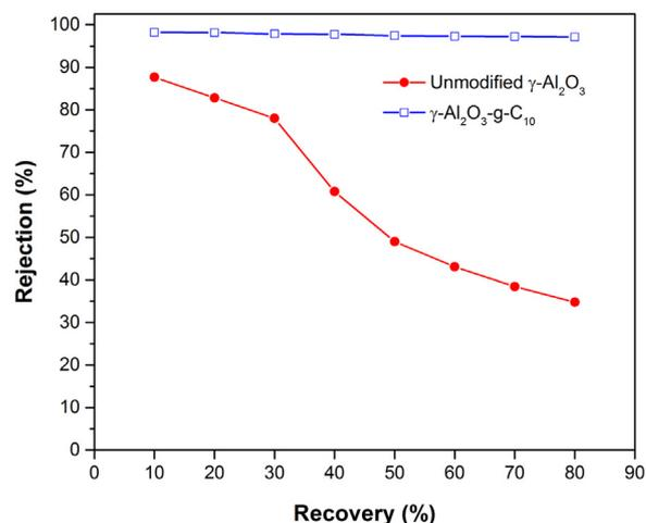
**Fig. 7.** SB rejection from toluene solution as function of recovery observed for unmodified and γ-alumina-g-C<sub>10</sub> membranes.
