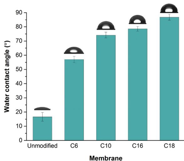
Fig. 4. Water contact angle of unmodified and grafted membranes.
