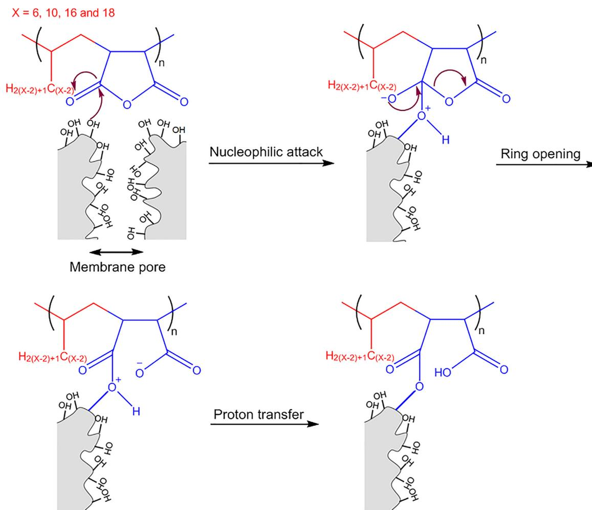
Fig. 1. Schematic diagram showing the grafting process of the alternating copolymers to  $\gamma$ -alumina membranes.
