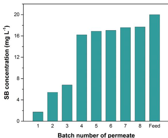
**Fig. 6.** SB concentrations from sample to sample for consecutive 20 ml batches of permeate for the unmodified membrane tested with 200 ml of SB/toluene.
