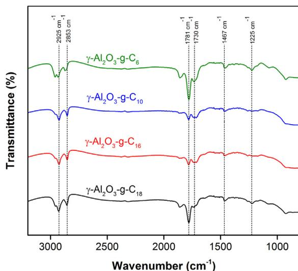
Fig. 2. FTIR spectra of the  $\gamma$ -alumina flakes grafted with different copolymers. The spectra were obtained by subtracting the spectrum of unmodified  $\gamma$ -alumina from each measurement.
