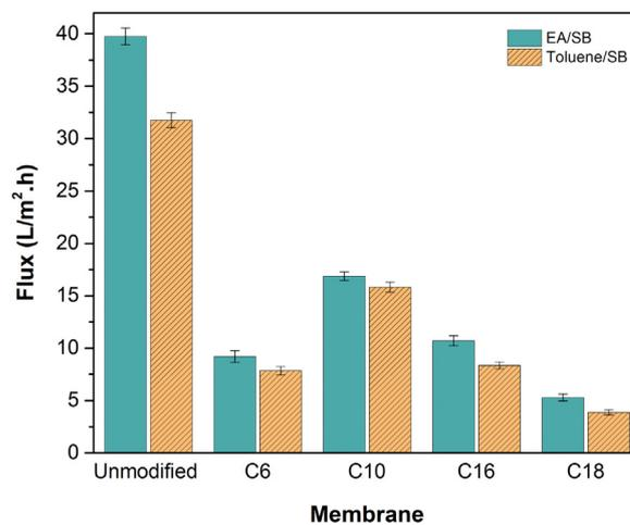
Fig. 5. Solvent flux of the unmodified and alternating copolymer-grafted  $\gamma$ -alumina membranes at TMP of 8 bar.
