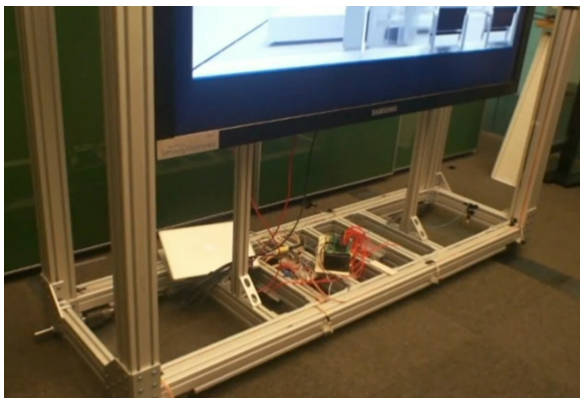
Fig. 17. Robotic sliding wall by MIT, frame on wheels (Larson, 2012)
