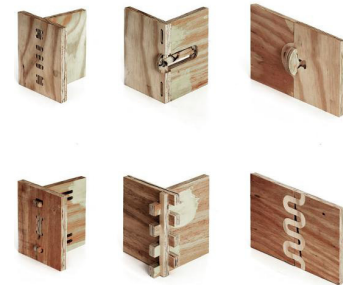
Fig 51. CNC-milled house and segment connections by Soutjesdijk (DeArchitect.nl, 2013)
