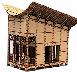
Fig 51. CNC-milled house and segment connections by Soutjesdijk (DeArchitect.nl, 2013)
