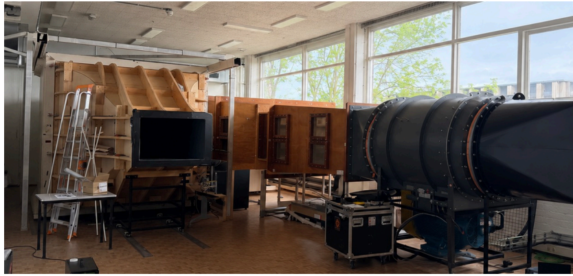
Figure 4.1: The Small Low-Turbulence Tunnel (SLT) in the Low Speed Lab at TU Delft. The axial fan and motor assembly are visible on the right, followed by the flow conditioning section housing the anti-turbulence screens. The contraction section (wooden structure, centre) accelerates the flow into the rectangular test section. The tunnel is shown in its open-loop configuration, without the test section present, before the measurement campaigns.
