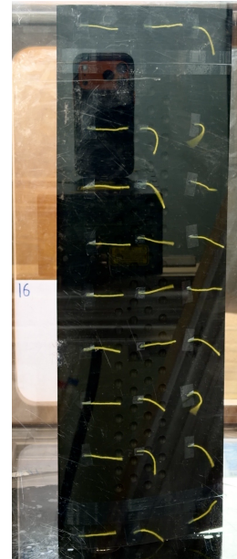
(b) Dimpled airfoil Mid-2.50 at \alpha = 16^\circ . Tufts at mid-span are nearly straight from leading to trailing edge, indicating attached flow. Separated cells are visible near each span end between x/c \approx 0.50 and the trailing edge, consistent with wall-junction end-effects.
