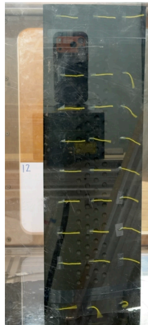
(b) Dimpled airfoil Mid-2.50 at \alpha = 12^\circ .
