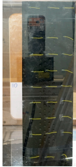
(b) Dimpled airfoil Mid-2.50 at \alpha = 10^\circ .
