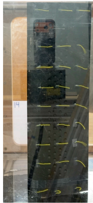
(b) Dimpled airfoil Mid-2.50 at \alpha = 14^\circ .
