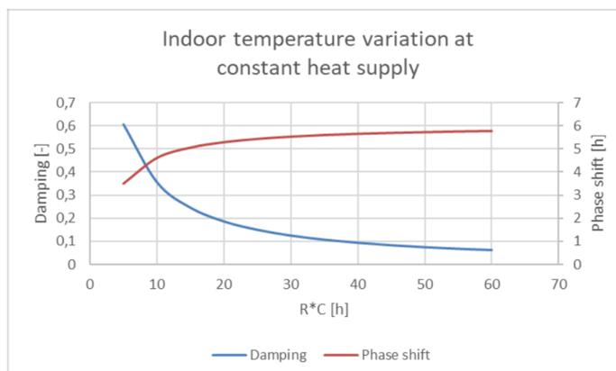
Figure E.1 – indoor variation at a fully load shifted thermal load profile (Memo on impact of maximum peak shaving on indoor temperature variation, n.d.)
