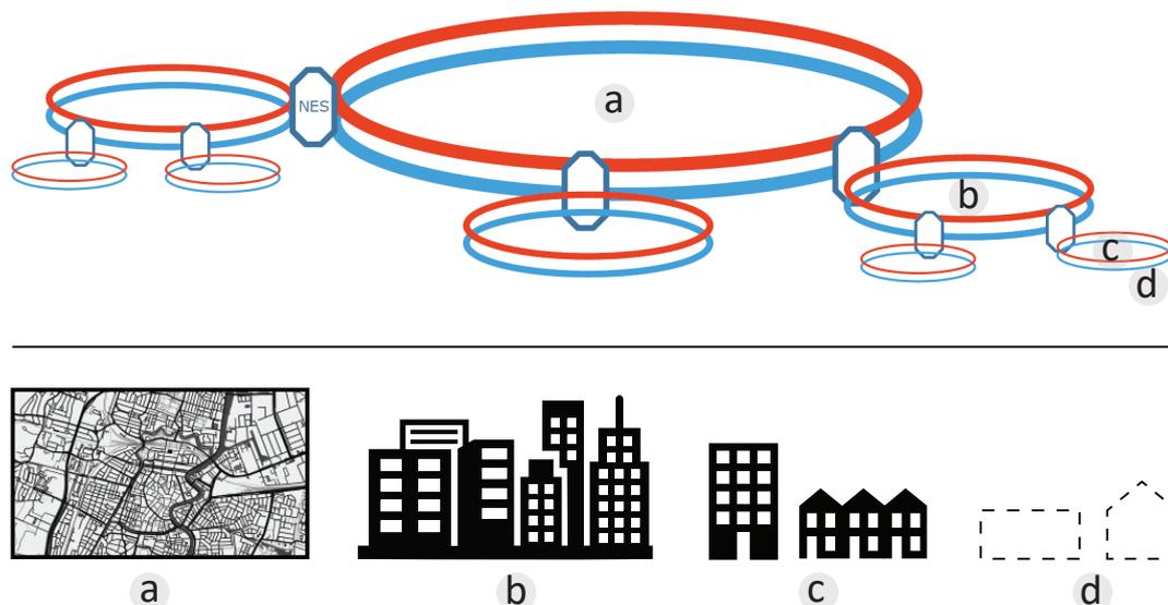
Figure 3.2 – The 5GDHC hierarchical levels: (a) the district or backbone, (b) urban block, (c) street and building unit level, adapted from (Jansen et al., 2019).
