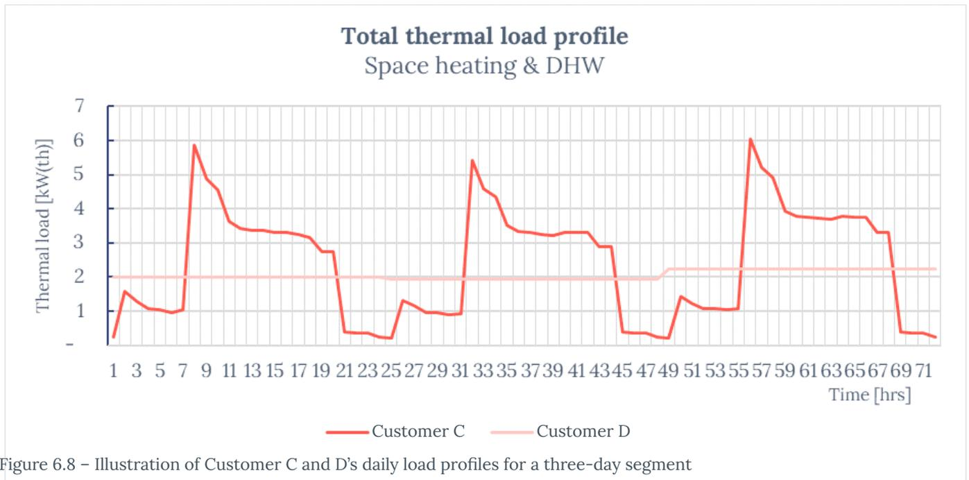
Figure 6.8 – Illustration of Customer C and D's daily load profiles for a three-day segment
