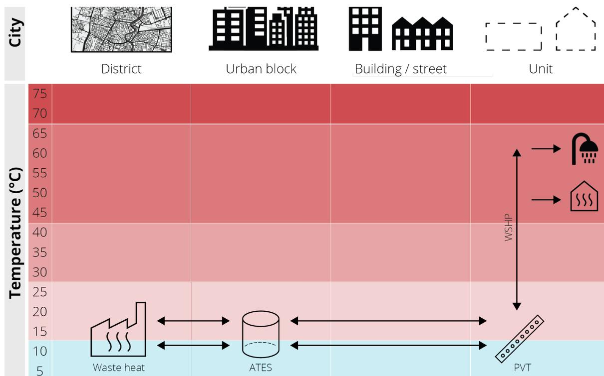
Figure 6.7 – The configuration of the test case with Waste heat as a secondary source
