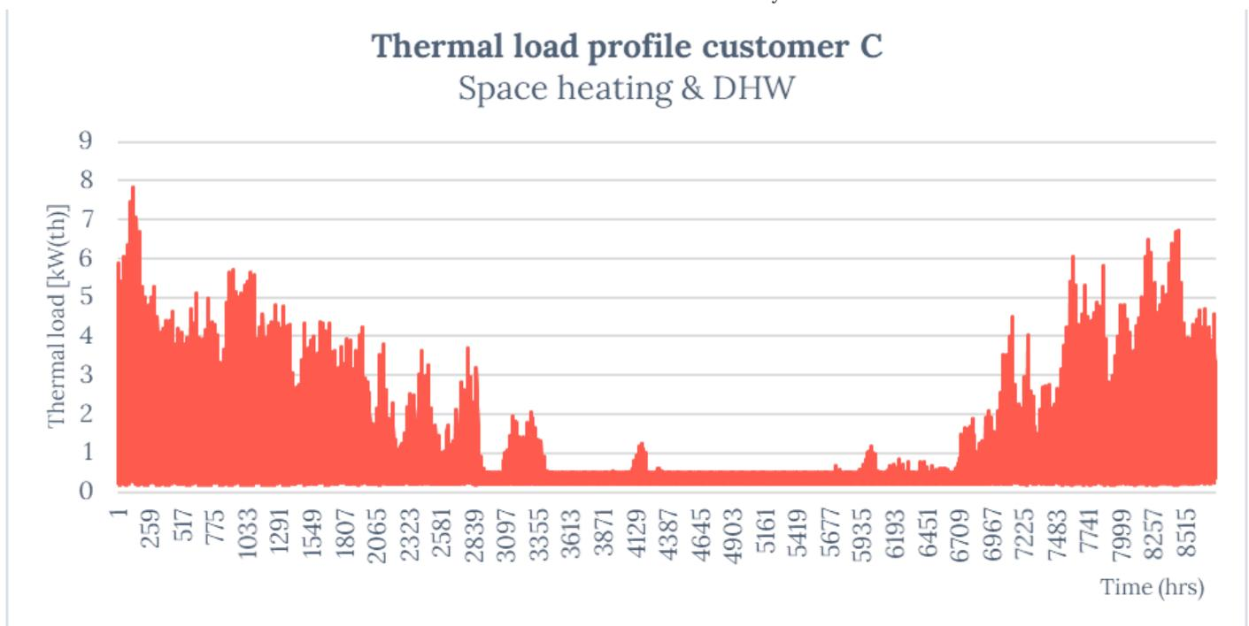
Figure 6.5 – One-year heat load profile for a single conventional customer type, adopted from received data DeZONNET Case (“DeZONNET Eindrapport”, Energy, 2020)
