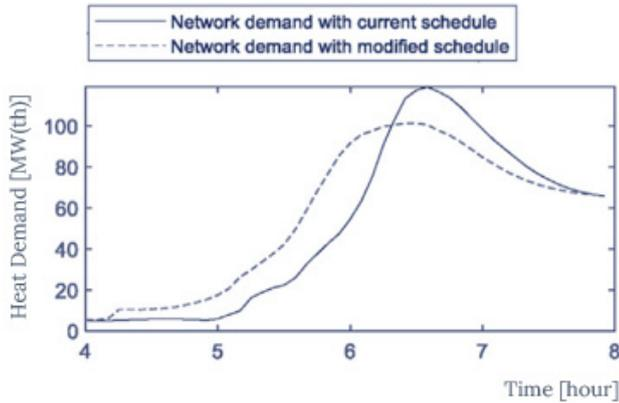
Figure 3.5 - An illustrative network thermal load profile before and after DSM: about 30% peak demand reduction (Guelpa & Verda, 2021).
