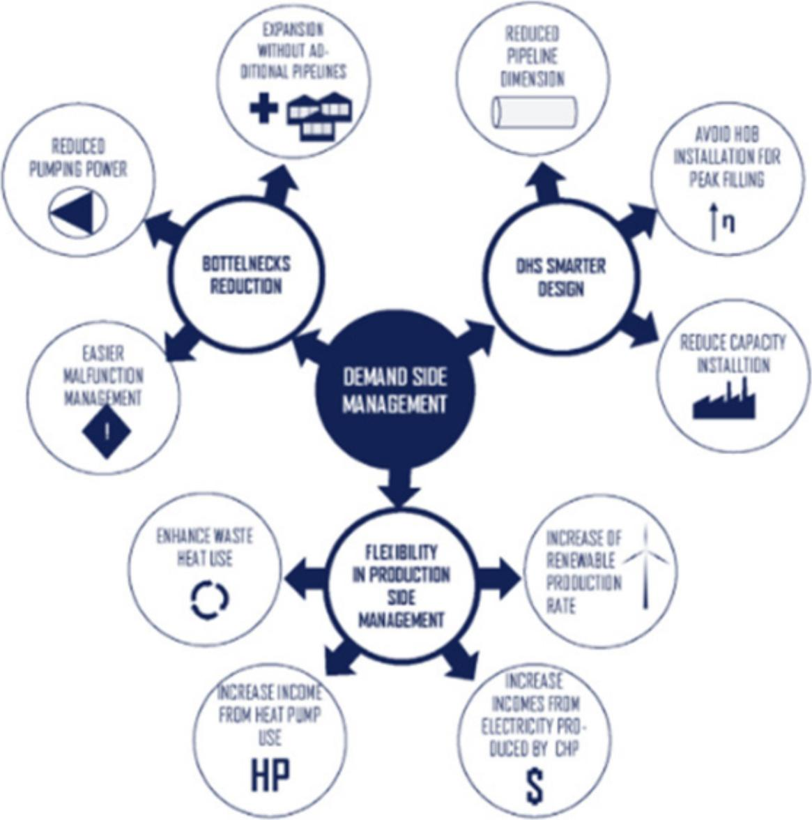
Figure D.1 - Schematic overview of the potential effects of DSM applications on DHC systems (Guelpa & Verda, 2019)
