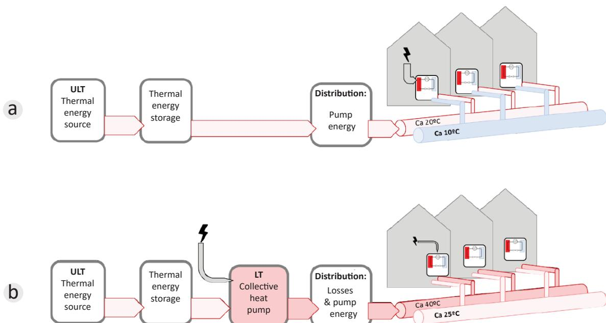
Figure 3.4 – (U)LT configurations and temperature levels at building level, adapted from (Jansen & Verhoeven, 2020)
