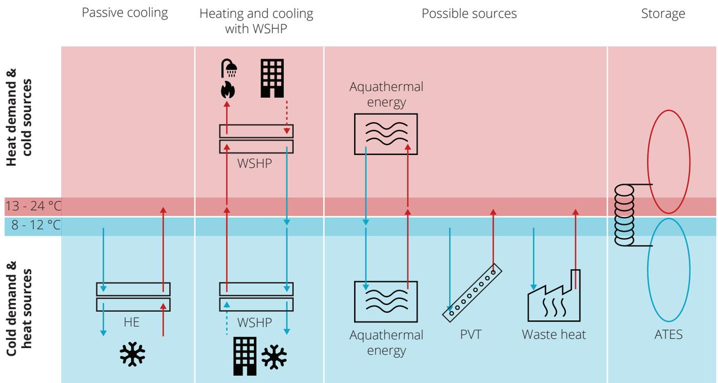
Figure 5.1 – A 5GDHC system configuration with typical operation and components as an example (Jansen & Verhoeven, 2020)
