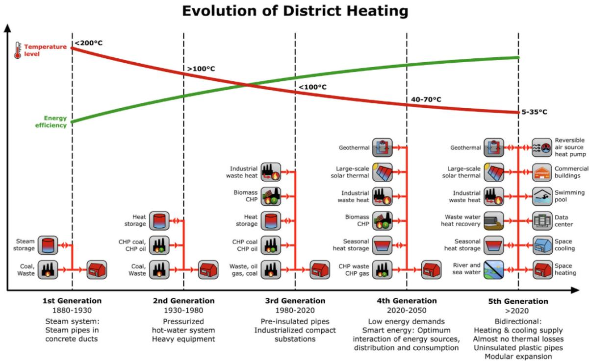
Figure 3.1 – Evolution of DH and DHC generations with 5GDHC as the latest available stage (Wirtz et. al, 2020a)
