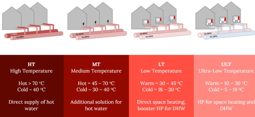
Figure 3.3 – Temperature levels in DH systems, adapted from (Jansen et al., 2019)
