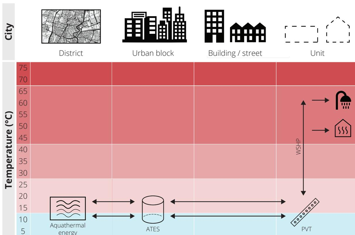
Figure 6.6 – The configuration of the test case with Aquathermal energy as secondary source
