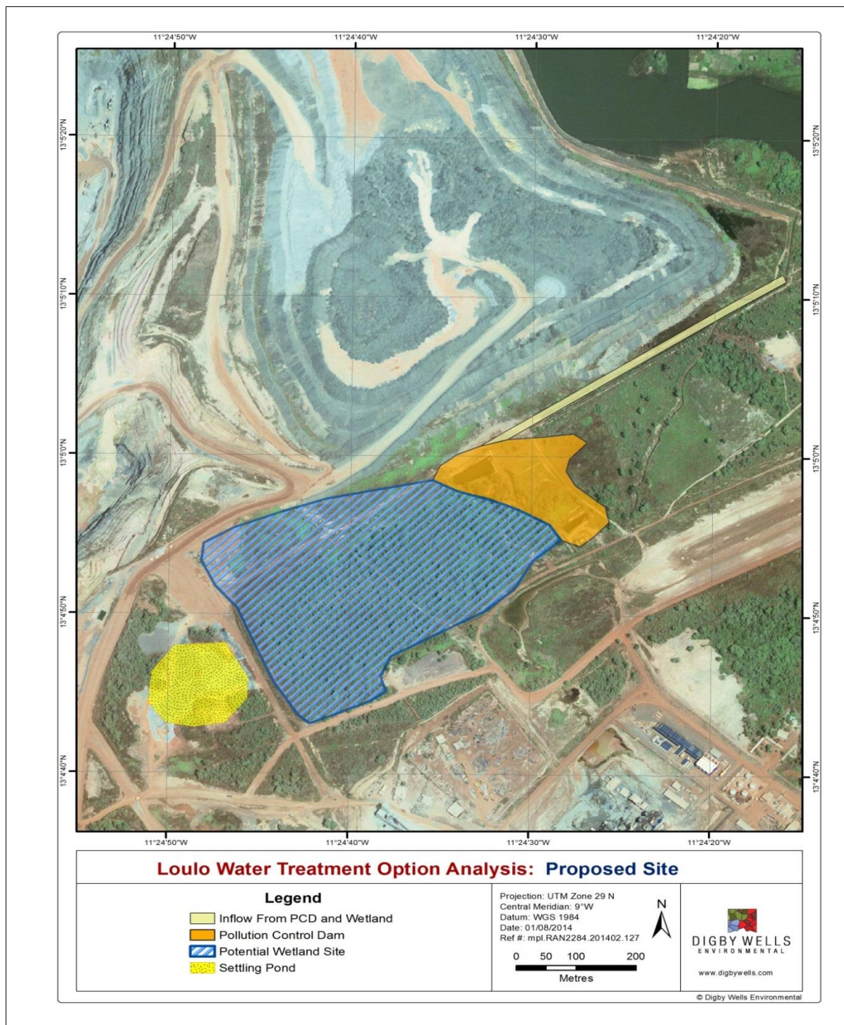
Figure 65. Illustration of the constructed wetland layout (Source: DWA, 2014)
