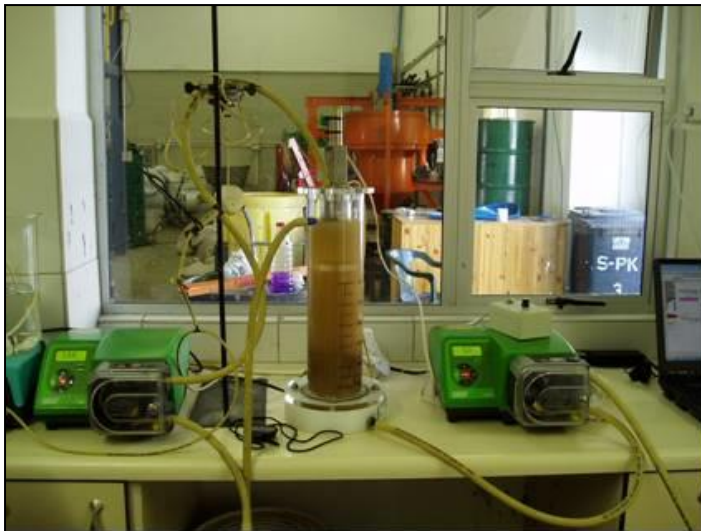
Figure 52. Bench-top dynamic thickening rig (P&C, 2011)
