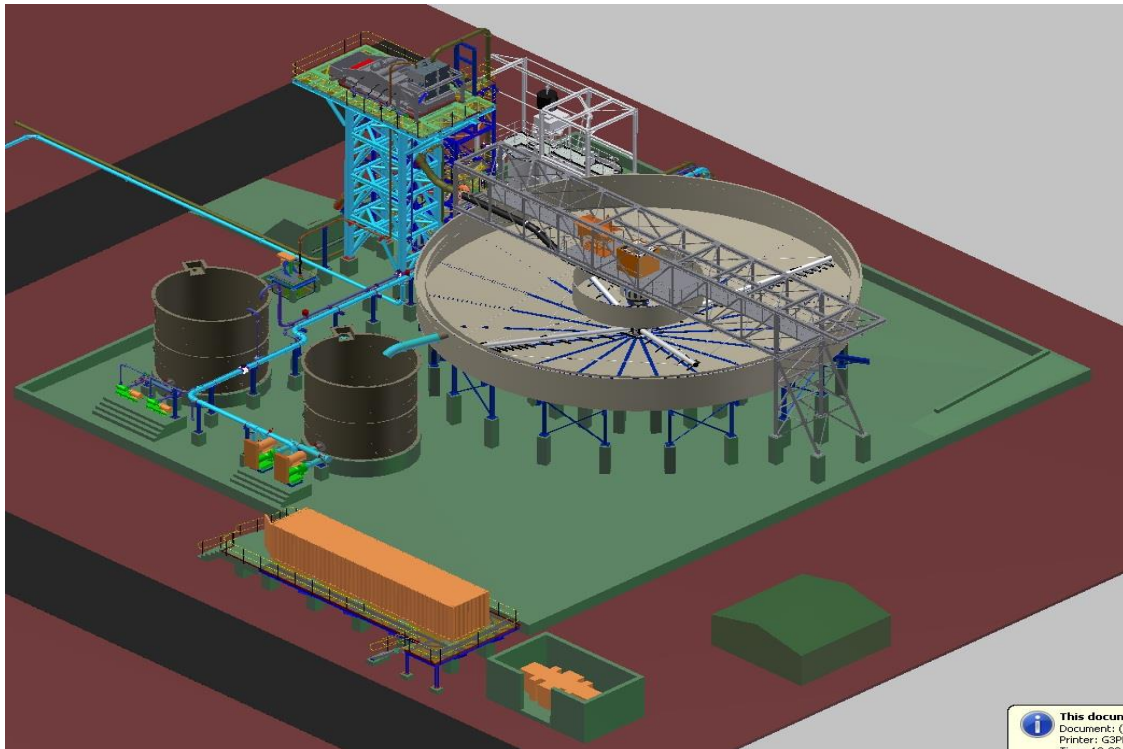
Figure 64. A 3D representation of the proposed thickener design (TWP, 2011)
