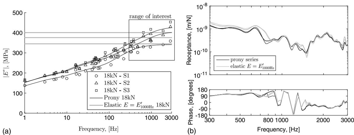
**Fig. 4.** New FC9 railpads at a toe load of 18 kN and a temperature of 26°C: (a) measured railpad dynamic properties (S: sample) and elastic and Prony series models; (b) simulated vertical track response
