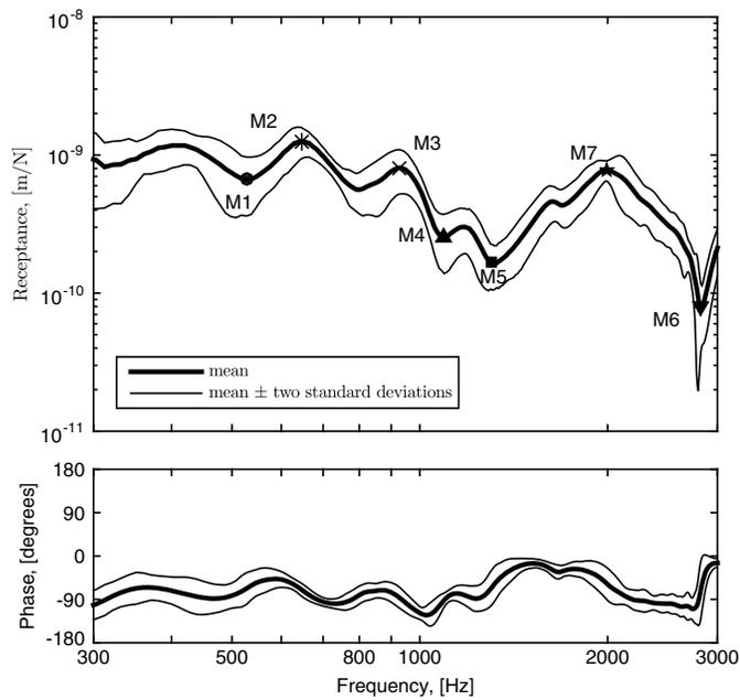
**Fig. 3.** Measured on-support track vertical receptance function; the characteristics are the second bending mode of the sleeper (M1), the in-phase rail resonance (M2), the antiphase rail resonance (M3), the pin-pin antiresonance (M4), the fourth bending mode of the sleeper (M5), the second-order pin-pin antiresonance (M6), and the 2,000 Hz resonance (M7)
