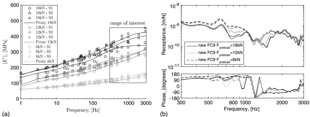
**Fig. 6.** New FC9 railpads at a temperature of 26°C for different toe loads, 18, 12, and 6 kN: (a) measured railpad dynamic properties (S: sample) and Prony series models; (b) simulated vertical track response
