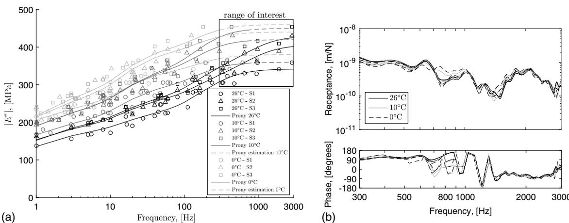
**Fig. 5.** New FC9 railpads for a toe load of 18 kN at different temperatures, 26, 10, and 0°C: (a) measured railpad dynamic properties (S: sample) and Prony series models; (b) simulated vertical track response
