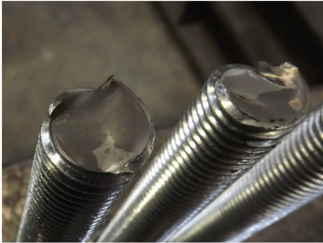
Fig. 15. Failure surface of bolts (P3.2-1).
