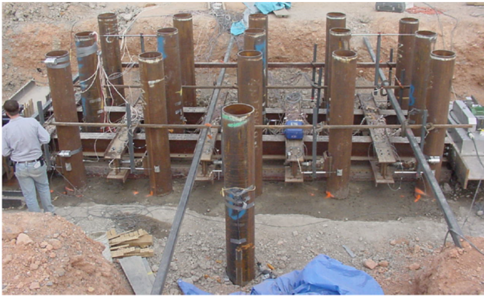
Figure A.4: Side view pile group loading test Salt Lake City case (Snyder, 2004), with left row being row 1
