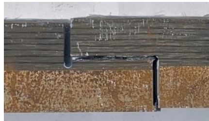
Figure 3.17: Failure behaviour of TAST 30-4
