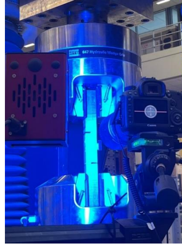
Figure 3.10: TASTs: surface that is measured by 2D DIC
