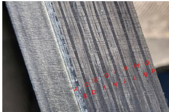
Figure 4.3: Laminate lay-up component samples
