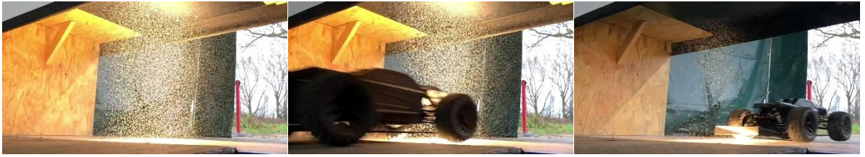
Figure 4. Illustration of the measurement domain before (left), during (middle) and after (right) the passage of the car.
