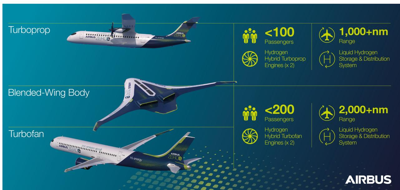
Figure 1.2: Airbus ZEROe concept aircraft. Source: adapted from [2].
