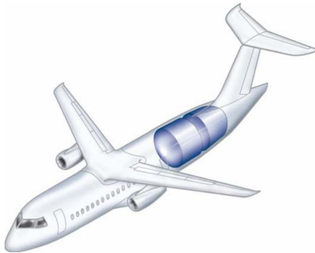
**Figure 2.3:** Small regional aircraft with aft tank<sup>1</sup>. Source: adapted from [5].
