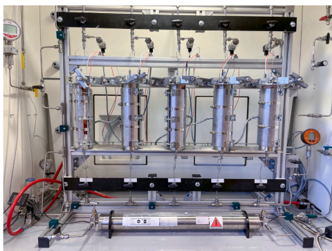
Fig. 2. Picture of the test system with 5 vertical autoclaves and piston cylinder (horizontal) for CO 2 feed.
