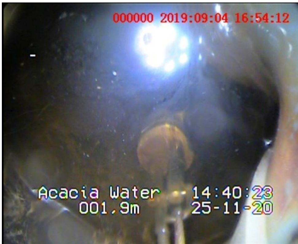
Figure 5.2: Metallic sheen on stagnant water within the standpipe taken November 25 th , 2020 after a 41-day standstill.
