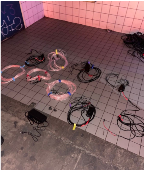
Figure 69 Color Coded Lights and Inverter Groups
