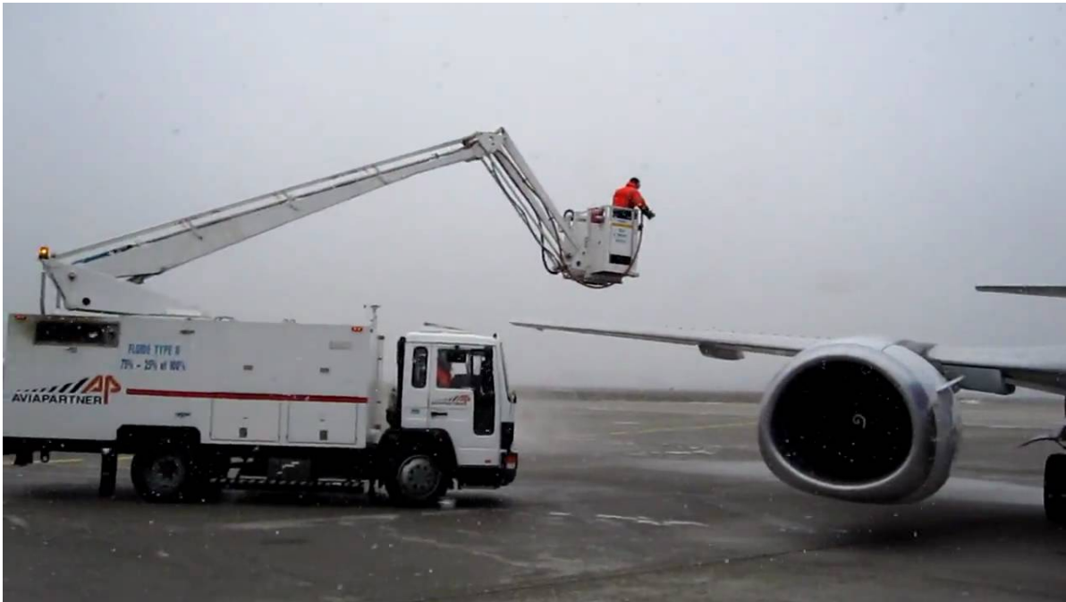
Figure 1.6: Deicing vehicle from the Aviapartner operation. Note that the deicing vehicle has an open basket, e.g. there is no cover protecting the worker in the basket. This deicing vehicle requires two people to operate: a driver and a deicer. (image taken as a still from https://youtu.be/5CP6grJi3AE )
