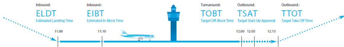
Figure 1.1: Five key CDM times graphically displayed. Two times for the inbound flight, and three for the outbound flight. Inbound is the process of the aircraft landing at the airport and taxiing to the gate. After the turn-around the aircraft becomes outbound, it leaves the airport. Image taken from [25]
