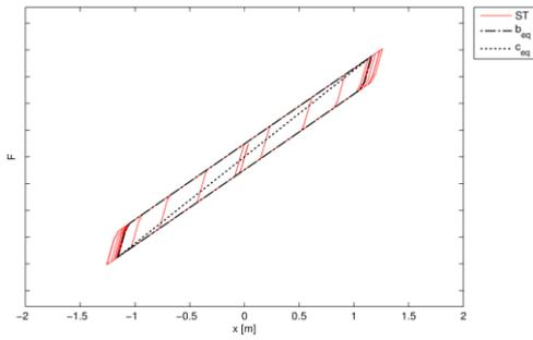
Figure 20: CS2 – Equivalent stiffness and damping
