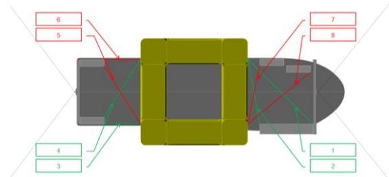
Figure 2: Mooring line configuration without ST
