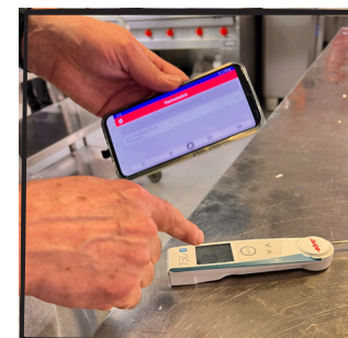
Sanitises the thermometer and connects to app via bluetooth
