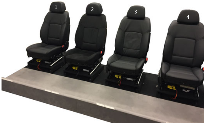
Fig. 1 The figure illustrates the setup of the study with all four seats in a row from left to right: reference seat ( seat 1 ); Alcantara seat ( seat 2 ); loose cover tension ( seat 3 ), and the seat with the metal plate instead of the seat suspension ( seat 4 )
