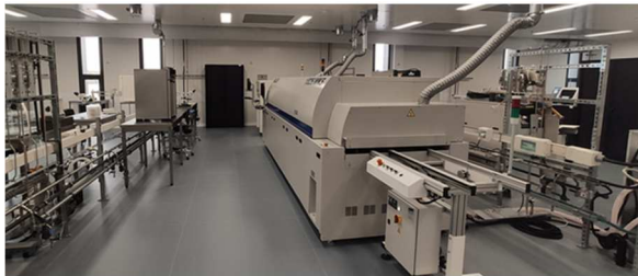
Figure 5 : Vernon's ISO7 clean room dedicated to ASIC integration
