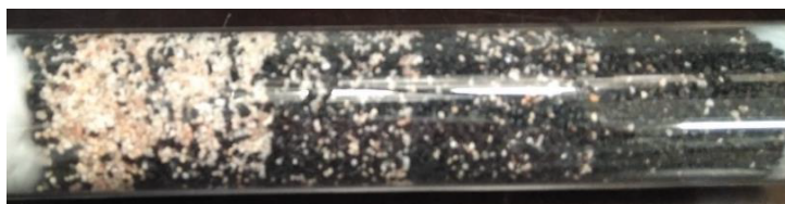
Figure 4.7: Photograph of the packed-bed, which consists of a mixture of progressively loaded activated carbon and quartz sand.
