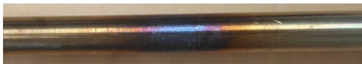
Figure 4.16: Tinted inner conductor due to oxidation after reaching temperatures around 600 °C.
