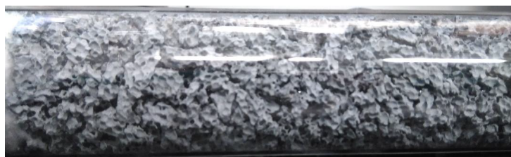
Figure 4.10: Crushed \alpha – SiC foam packed bed.
