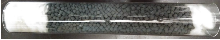
Figure 4.12: Microwave active bed of \beta – SiC extrudates of 5 mm lumped size
